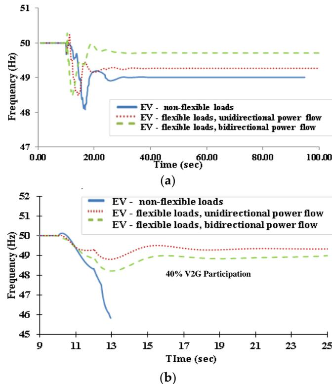
**Figure 6.** Simulation of (a) a three-phase short circuit at a high-voltage bus and (b) a three-phase short circuit at a high-voltage bus with simultaneous loss of two generators in the Greek non-interconnected island of Crete [16].
