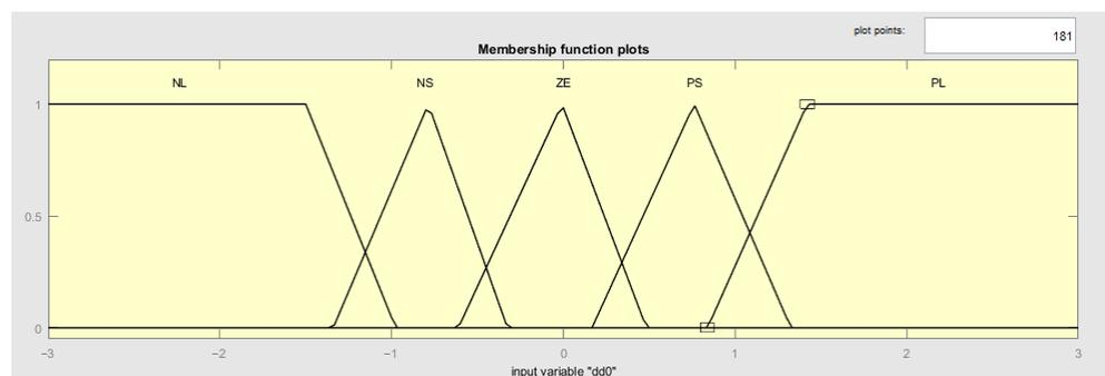
Figure 9. Membership functions of the input variable “power gradient”.
