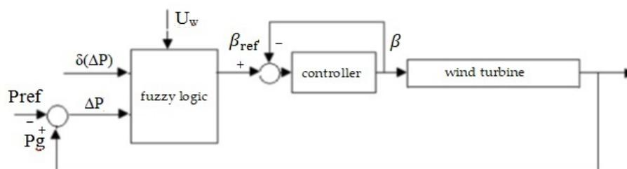
Figure 1. A block diagram of a controller with an algorithm based on fuzzy logic for changing the pitch angle blade of the wind turbine.
