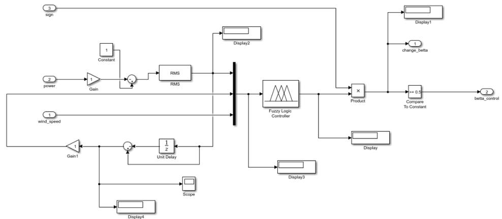
Figure 7. Pitch angle change block in MATLAB.
