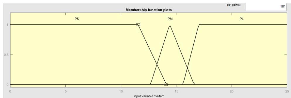
Figure 10. Membership functions of the input variable “wind speed”.
