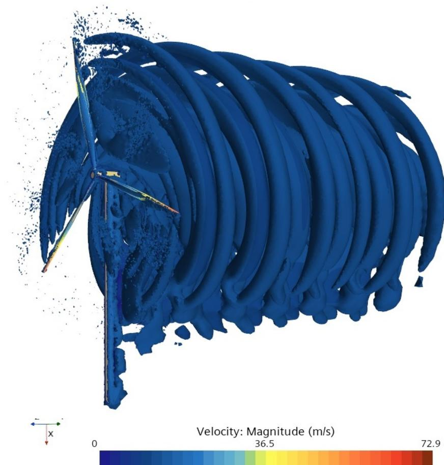
Figure 13. Wind turbine near wake display scene.
