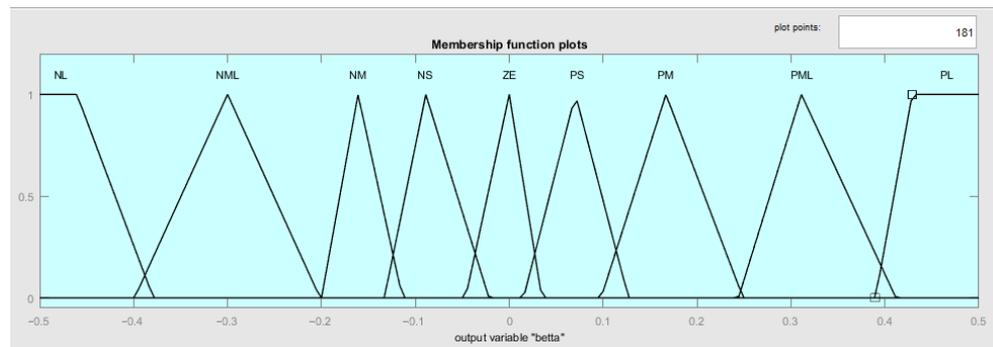
**Figure 11.** Membership function of the output value “blade pitch angle”.
