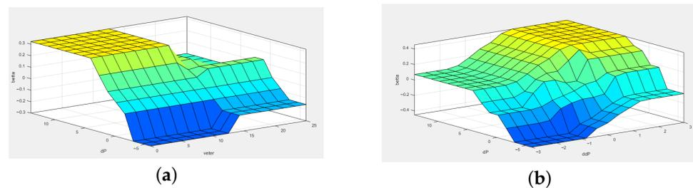
**Figure 12.** The surface of the algorithm defuzzification results depends on: (a) power deviation, pitch angle and wind speed; (b) pitch angle, power deviation and power deviation error.
