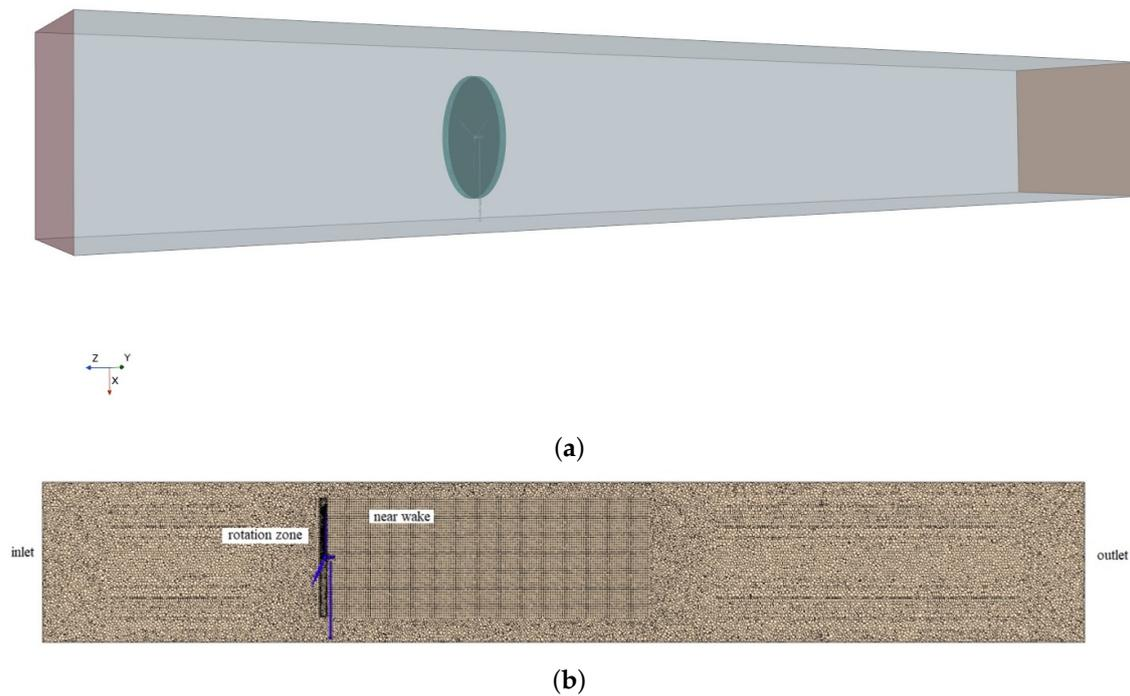
**Figure 2.** (a) Calculation area of the wind generator and (b) mesh for modeling a wind turbine.
