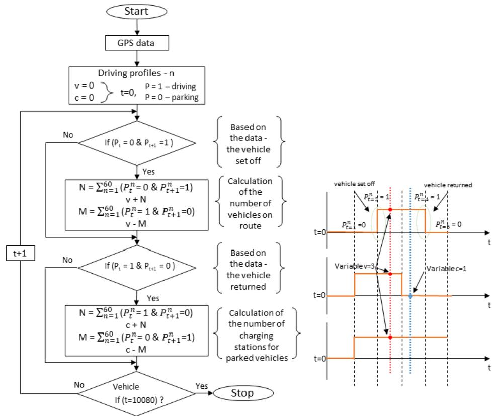
Figure 14. Block diagram of the algorithm implemented.
