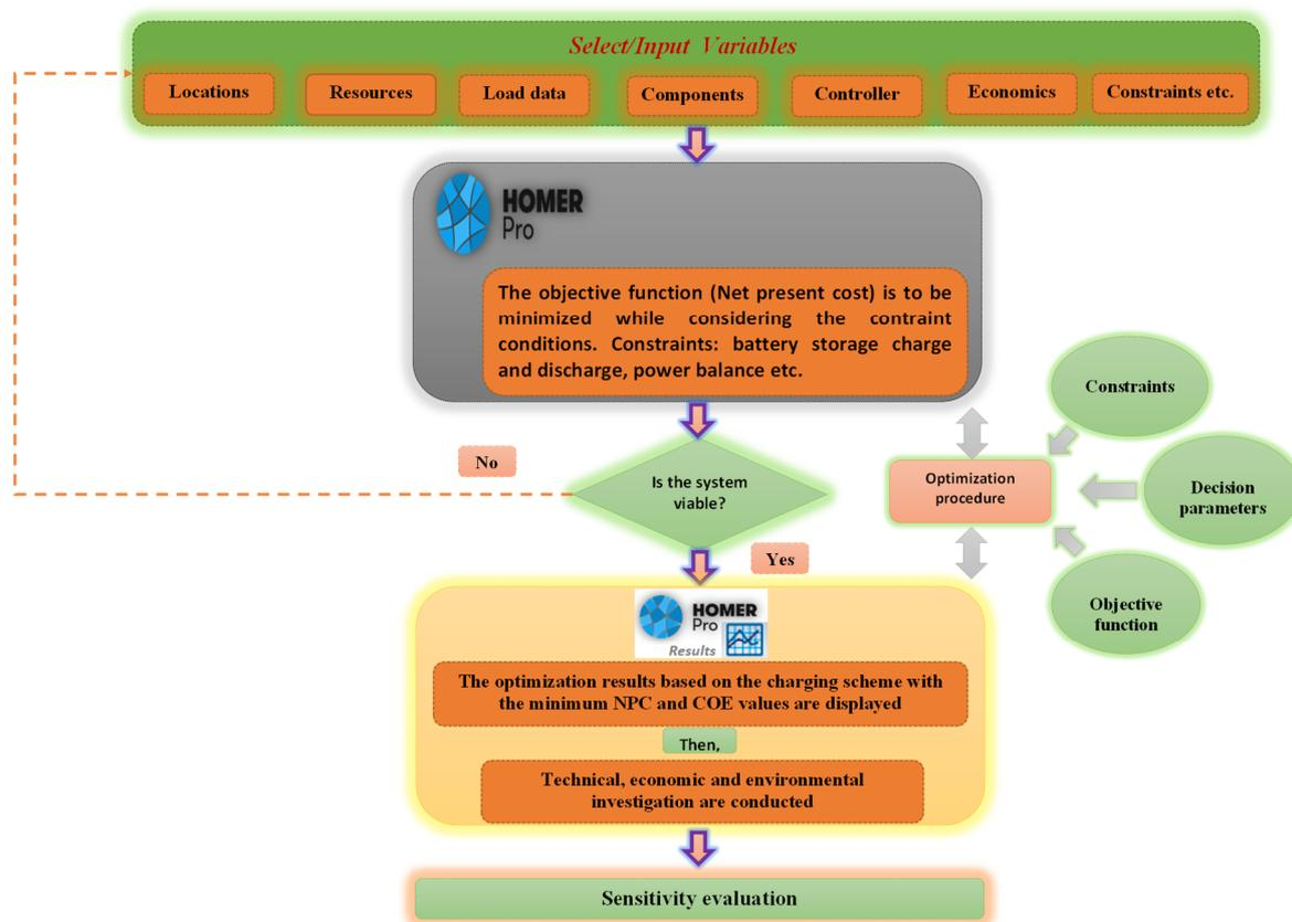
**Figure 4.** Assessment flowchart and optimization process utilized in the HOMER Pro<sup>®</sup> microgrid tool.
