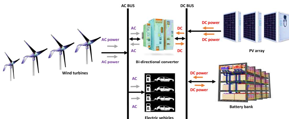
Figure 3. The energy flow schematic diagram of the suggested hybrid RE-based charging stations.
