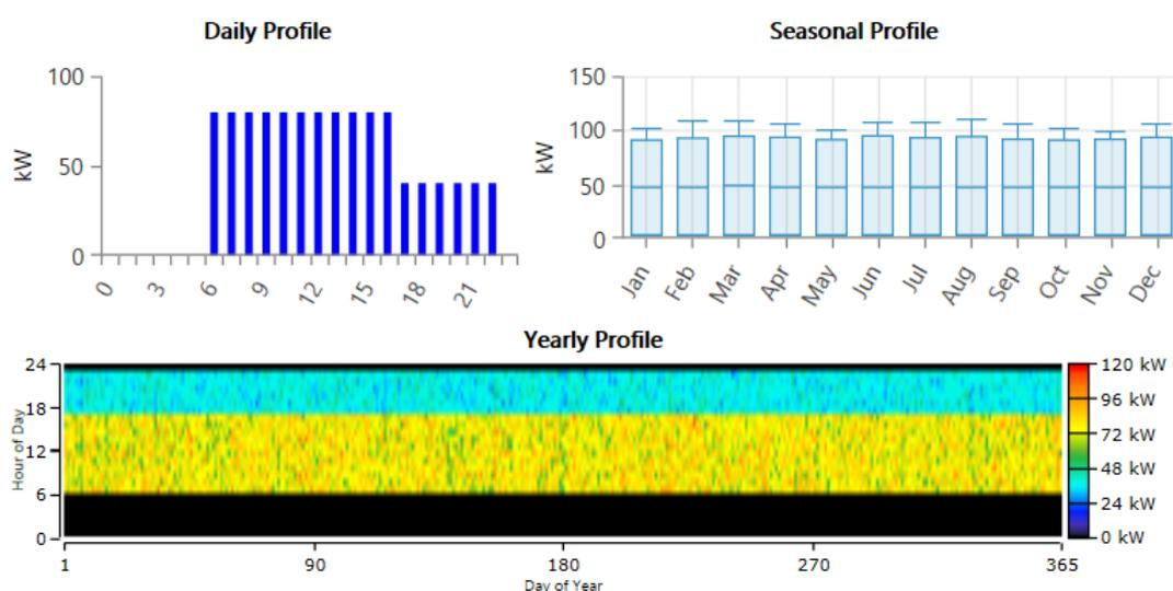
Figure 6. EV charging station system load profile.
