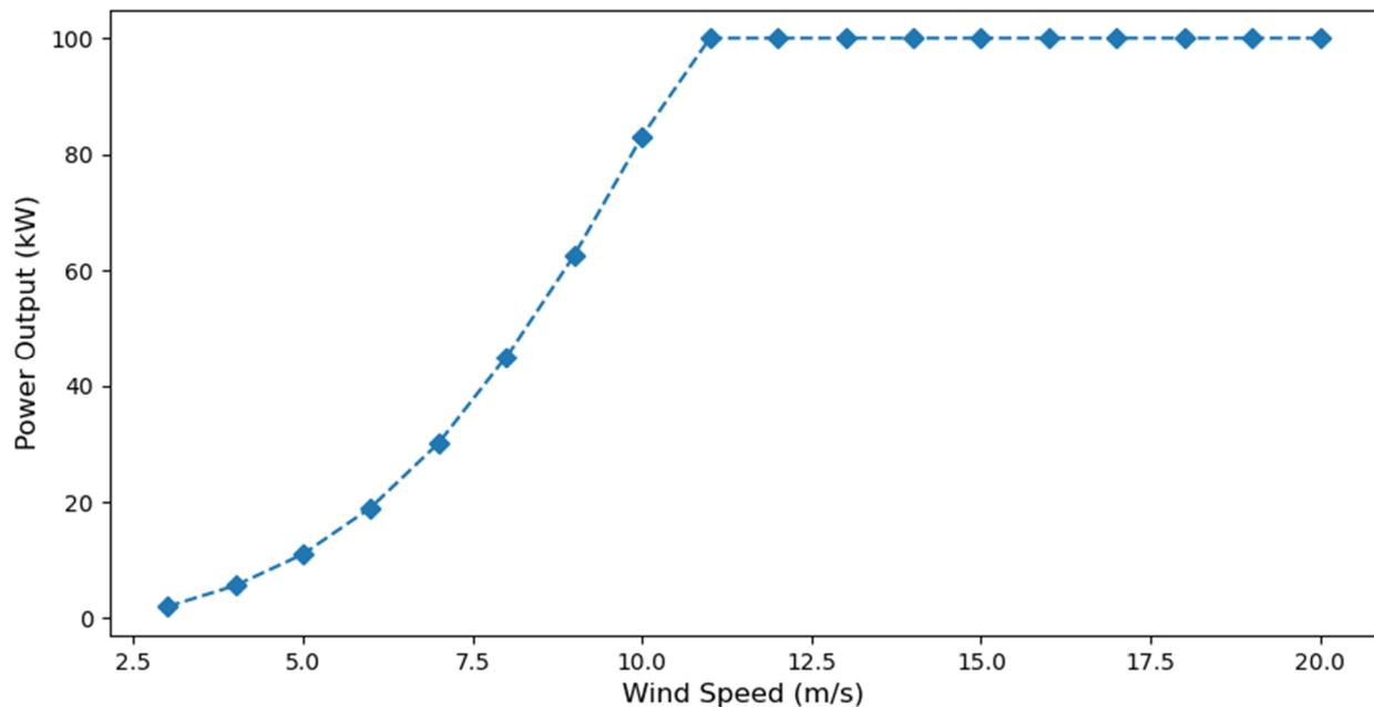
**Figure 5.** The WT power curve.
