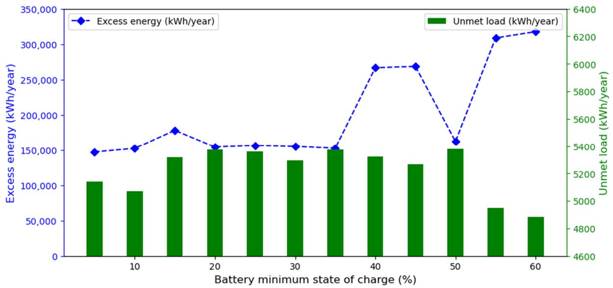
Figure 17. The effect of varying the battery SOC<sub>minimum</sub> percent value on the technical performance of the optimal charging system.
