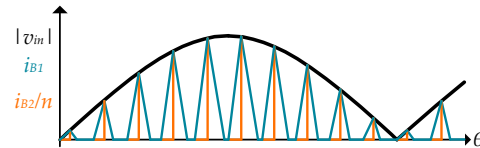
Figure 5. DAB input and output currents evolution with the rectified input voltage. In black rectified ac mains, in blue is the current of rectified ac mains, and in orange is the rectified secondary current of the DAB.
