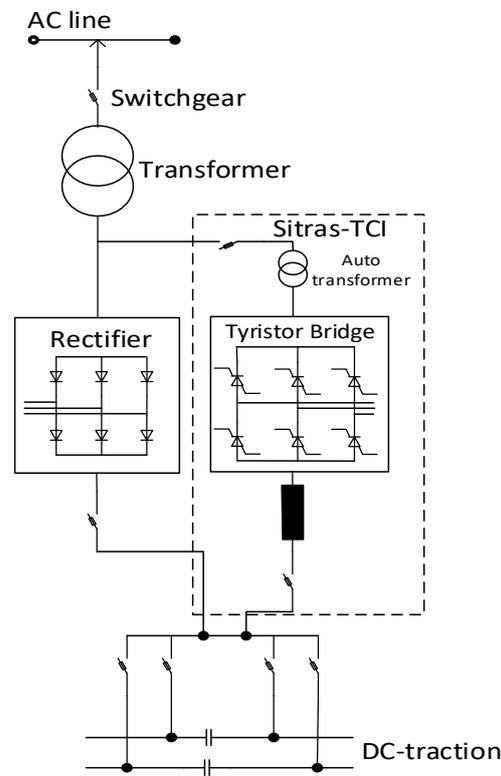
Figure 15. Siemens Sitras-TCI substation.
