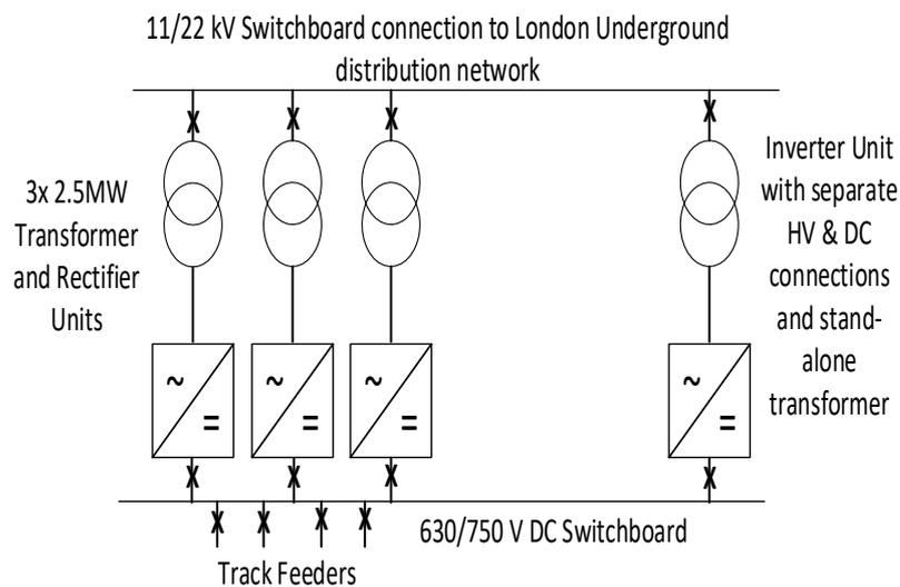
Figure 20. Upgraded version of the traction system of the London Underground [128].
