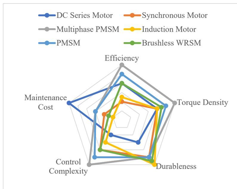
**Figure 10.** Spider web comparison chart of traction motors.
