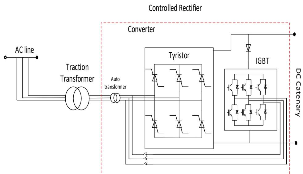
Figure 18. Improved HESOP converter by SNCF [126].
