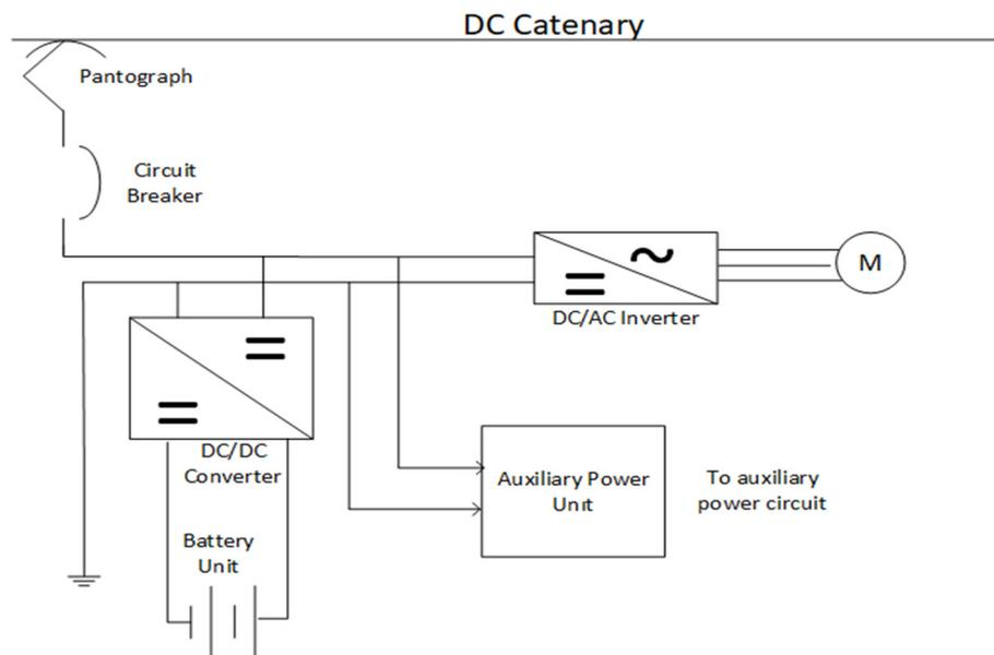
**Figure 1.** Electric with battery traction system [20].
