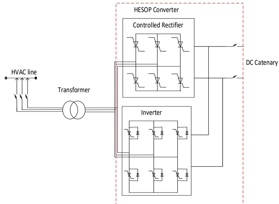
Figure 17. Harmonic and energy-saving optimizer (HESOP) converter [101].
