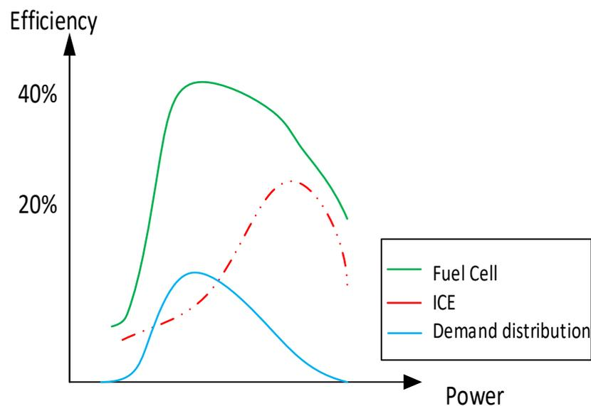
**Figure 7.** Fuel Cell & ICE Power Efficiency Curves [41].
