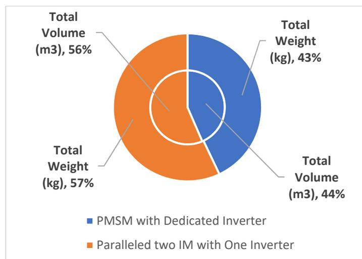
Figure 9. Overall volume and weight comparison.
