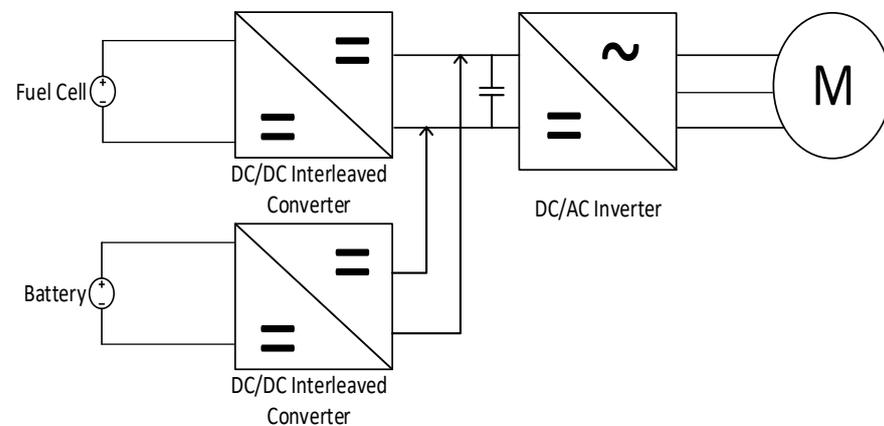
**Figure 6.** Fuel cell–battery hybrid traction [19].
