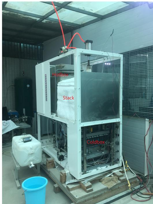
**Figure 1.** Physical diagram of 1kW SOFC power generation system.
