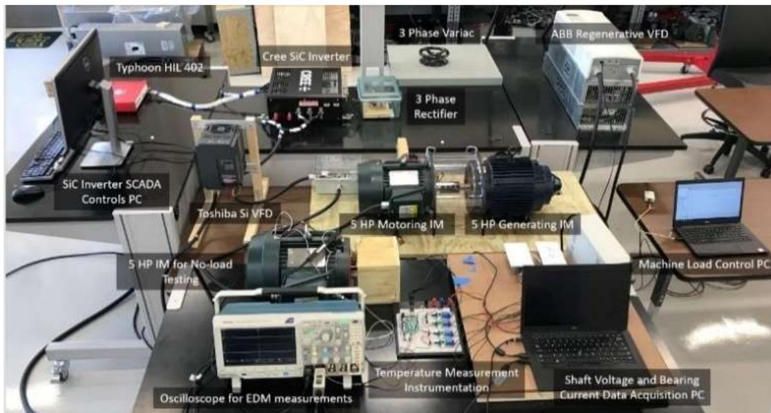
**Figure 6.** Experimental testbed constructed for the acquisition of shaft voltages and EDM bearing currents for Si- and SiC-based PWM inverters.
