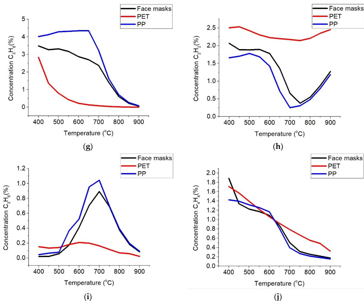
**Figure 8.** Influence of temperature on formation of (a) CO, (b) H<sub>2</sub>, (c) CH<sub>4</sub>, (d) C<sub>6</sub>H<sub>6</sub>, (e) C<sub>2</sub>H<sub>4</sub>, (f) C<sub>2</sub>H<sub>6</sub>, (g) C<sub>3</sub>H<sub>8</sub>, (h) C<sub>2</sub>H<sub>2</sub>, (i) C<sub>3</sub>H<sub>6</sub>, (j) C<sub>4</sub>H<sub>4</sub>.
