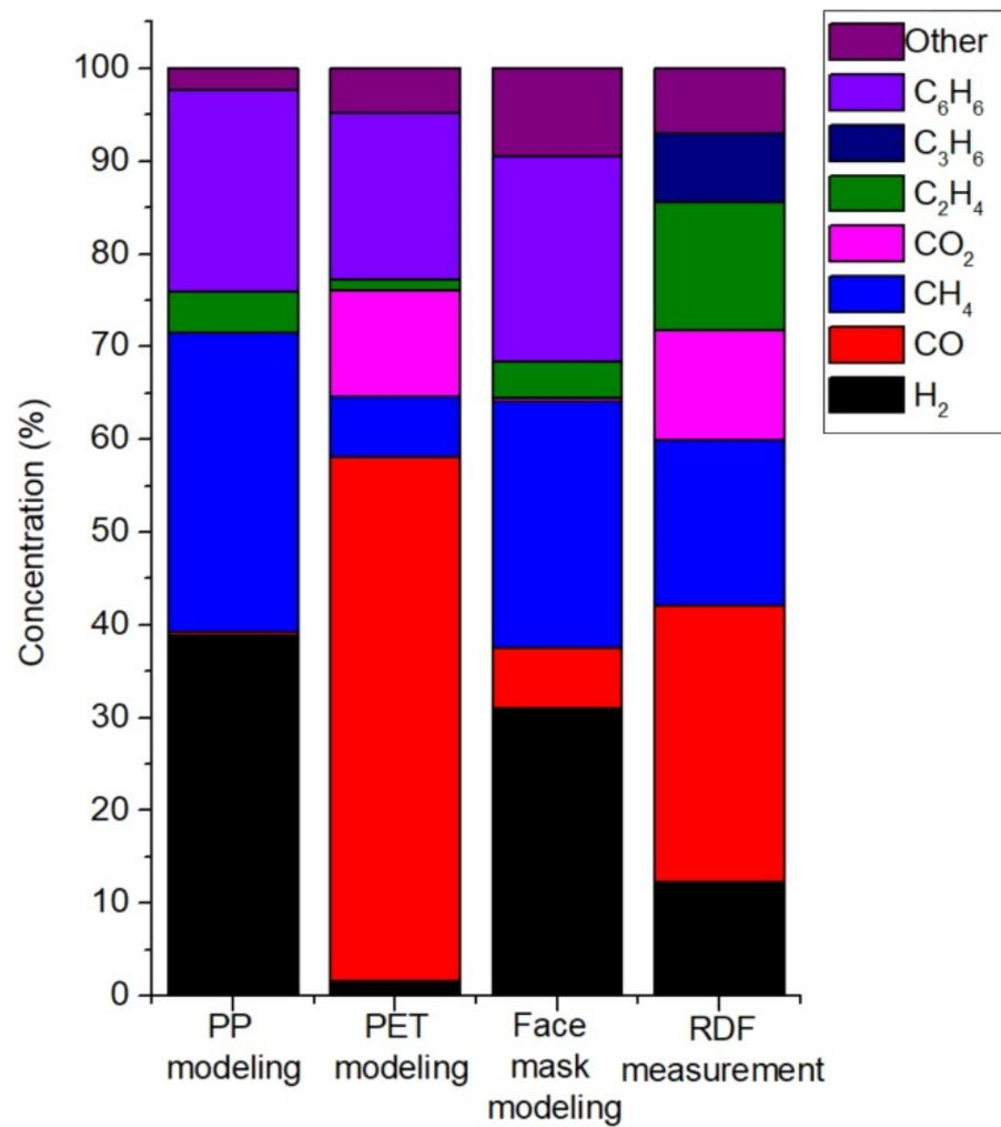
Figure 9. Comparison of selected gaseous pyrolysis products.
