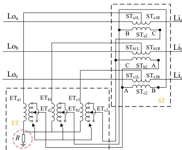
Figure 3. Structure of a phase-shifting and grounding transformer (PSGT).
