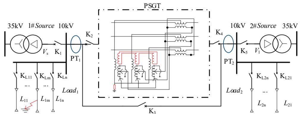
Figure 7. A single-phase ground fault scene occurred in a cable of the distribution network.
