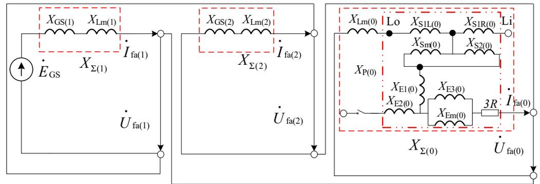
Figure 8. Composite sequential network diagram.
