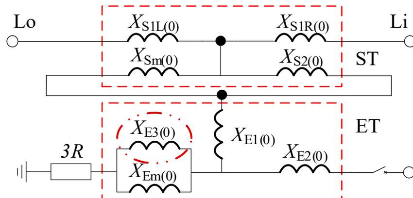
Figure 6. Zero-sequence equivalent circuit after adding windings.
