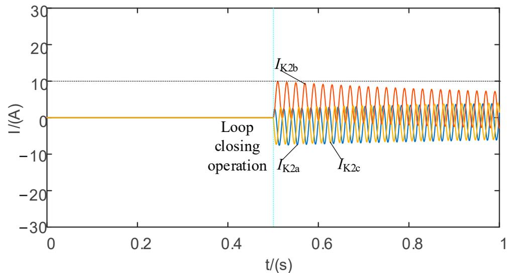
**Figure 9.** Loop closing current flowing through  $K_2$ .
