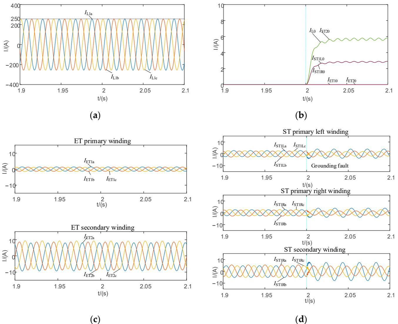
**Figure 10.** This is based on the PST loop closing device and a fault current. (a) Bus 1# three-phase current; (b) Faulted line and closing loop device zero-sequence current; (c) Excitation transformer (ET) each winding three-phase current; (d) Series transformer (ST) each winding three-phase current.
