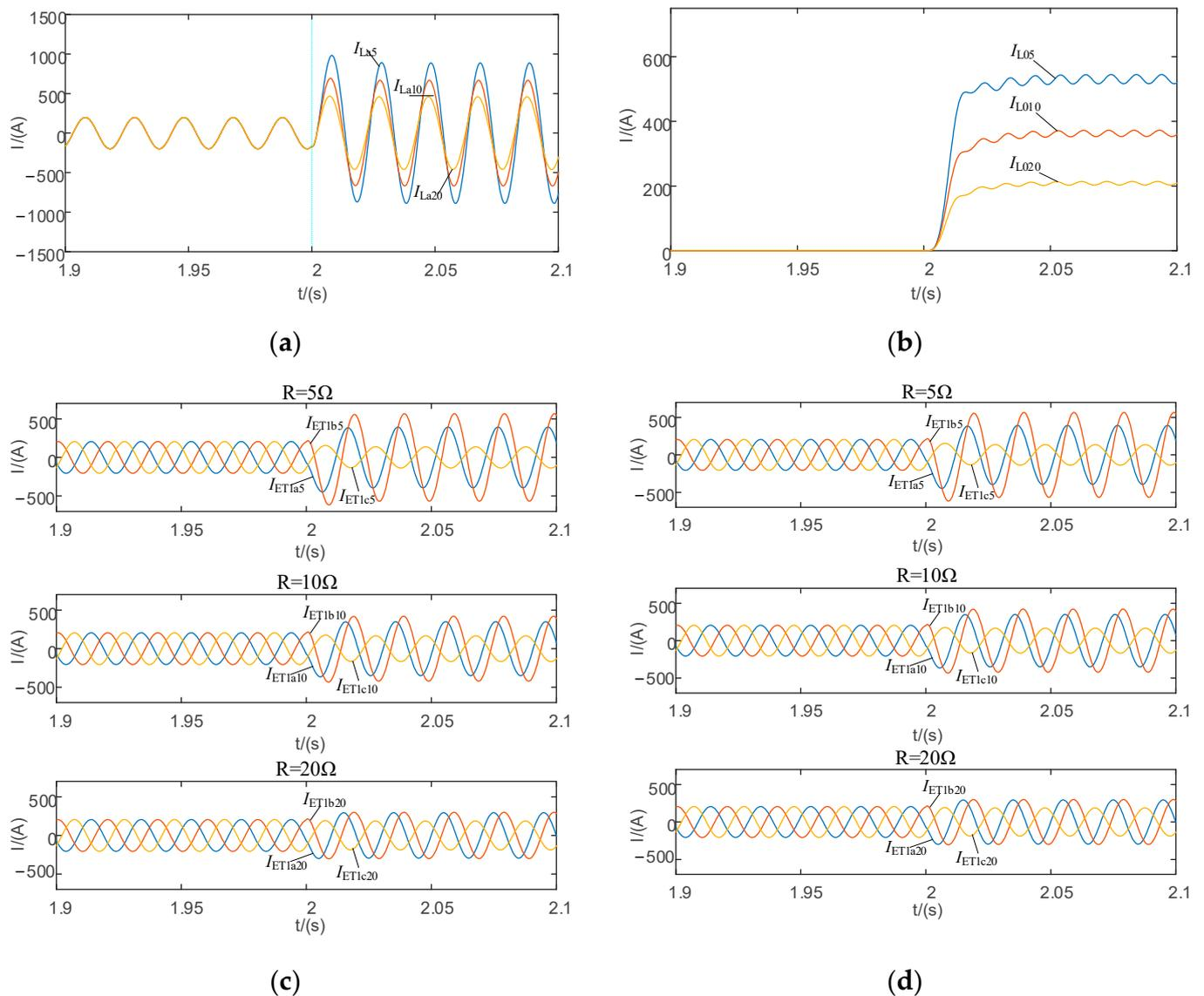
**Figure 12.** This is based on a different ground resistance PSGT and fault line current. (a) Bus 1# fault phase current; (b) Zero sequence current of the faulty line; (c) ET primary winding three-phase current; (d) ST primary winding three-phase current.
