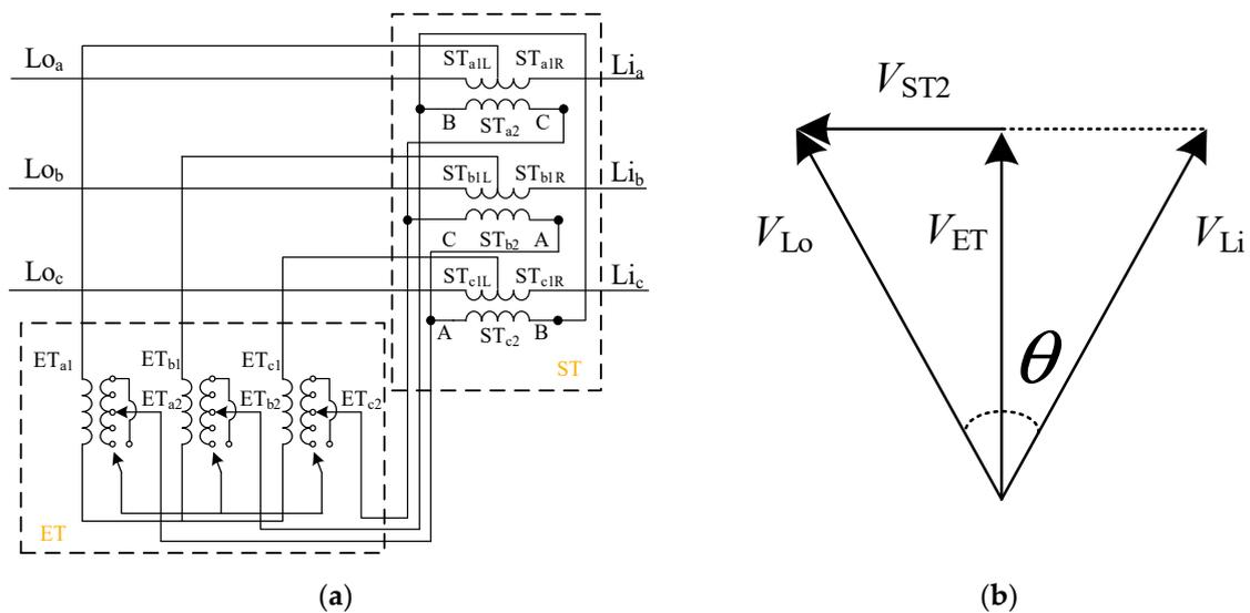
Figure 2. (a) Structure of double-core symmetrical PST; (b) Regulation vector diagram of a PST.
