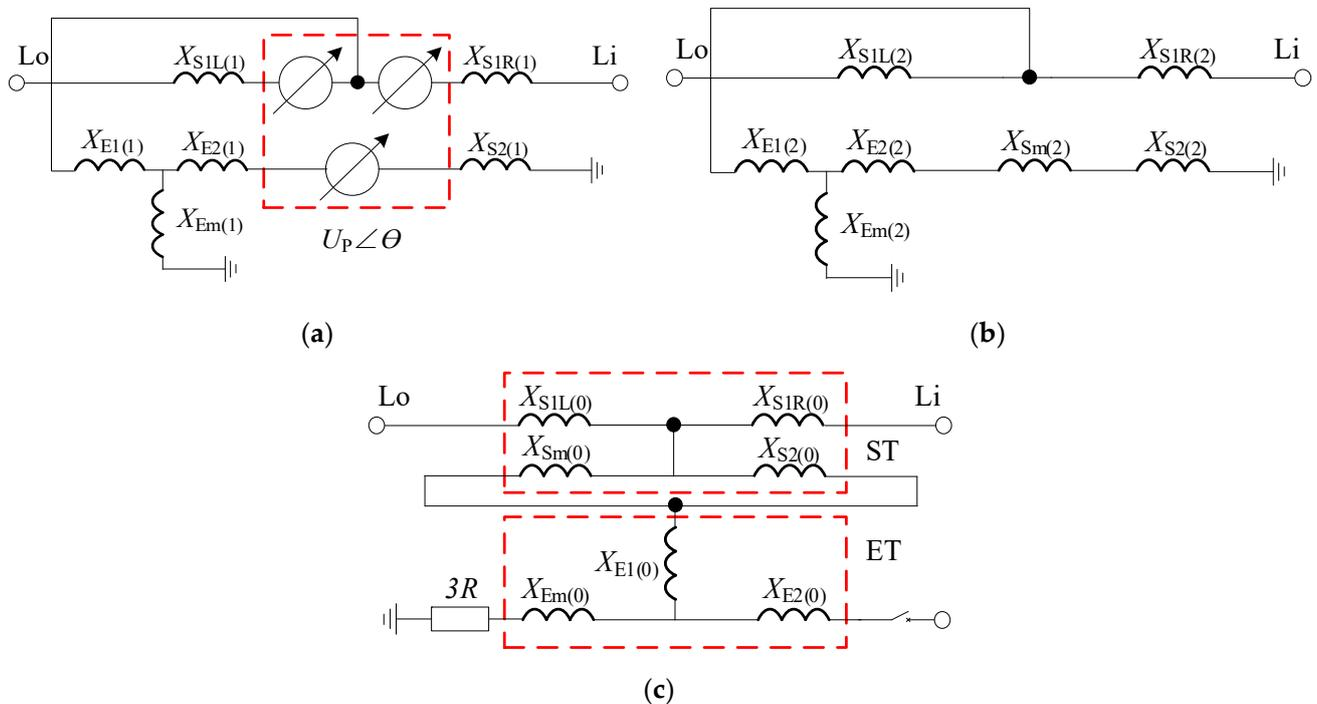
**Figure 4.** This is the phase-shifting and grounding transformer three-sequence equivalent circuit. (a) Positive sequence equivalent circuit; (b) Negative sequence equivalent circuit; (c) Zero sequence equivalent circuit.
