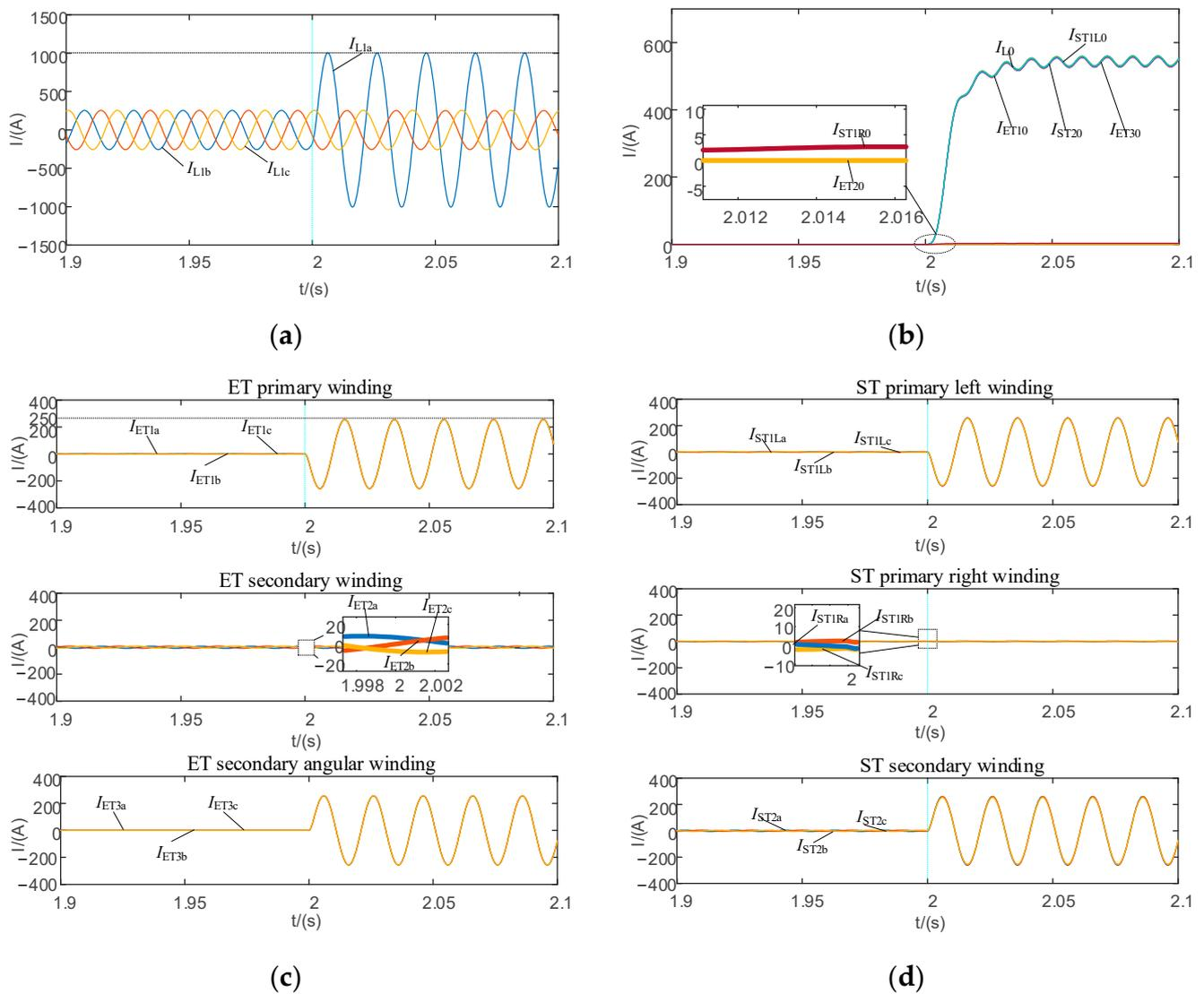
**Figure 11.** This is based on the PSGT loop closing device and fault current. (a) Bus 1# three-phase current; (b) Faulted line and closing loop device zero-sequence current; (c) ET each winding three-phase current; (d) ST each winding three-phase current.
