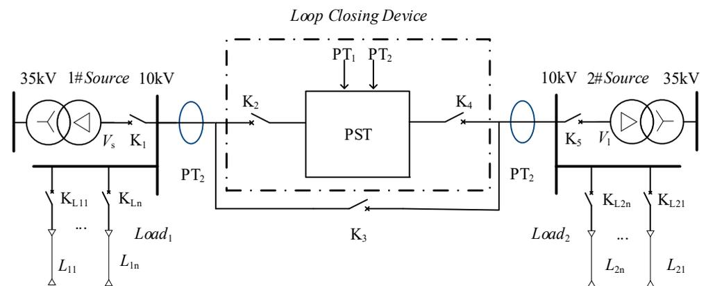
**Figure 1.** Application scenarios of a phase-shifting transformer (PST).
