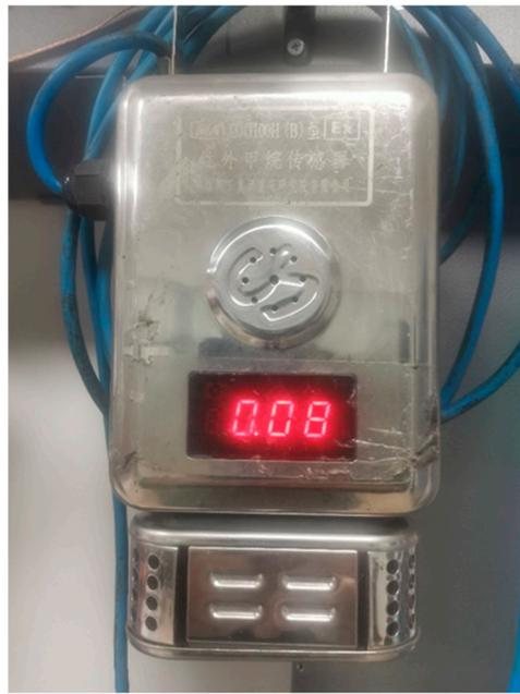
**Figure 1.** Methane transducer.
