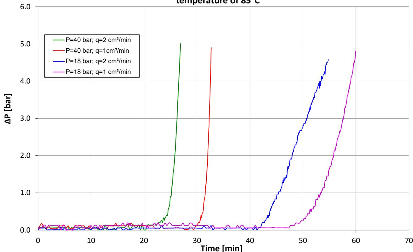
**Figure 4.** Tests for the precipitation of sediments for water "A" modified with sodium bicarbonate (2 g/800 mL) and water "B" at a temperature of 85 °C (measurement error is  $\pm 4\%$ ).
