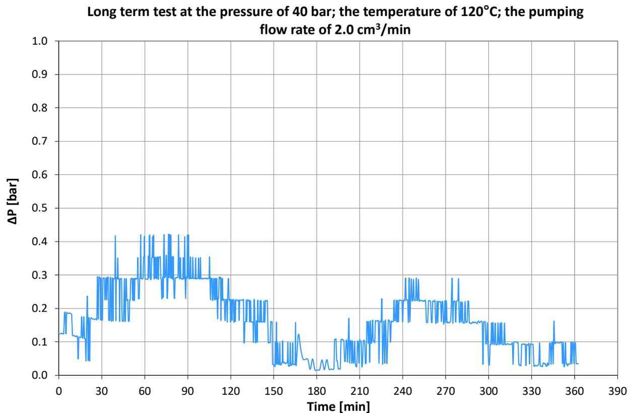
**Figure 8.** Long-term test of waters “A” and “B” under the following conditions:  $P = 40$  bar,  $T = 120$  °C and  $q = 2.0$  cm<sup>3</sup>/min for each of the brine types (measurement error is  $\pm 4\%$ ).
