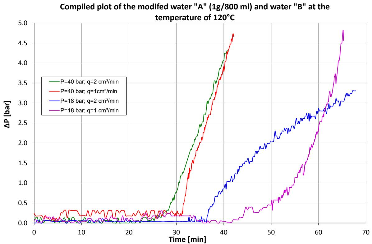
**Figure 7.** Tests for the precipitation of sediments for water “A” modified with sodium bicarbonate (1 g/800 mL) and water “B” at a temperature of 120 °C (measurement error is  $\pm 4\%$ ).
