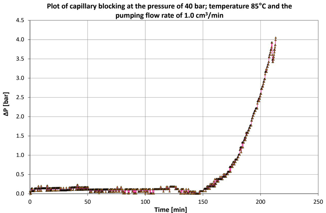
**Figure 6.** Tests for the precipitation of sediments for water “A” modified with sodium bicarbonate (1 g/800 mL) and water “B” at a temperature of 85 °C (measurement error is  $\pm 4\%$ ).
