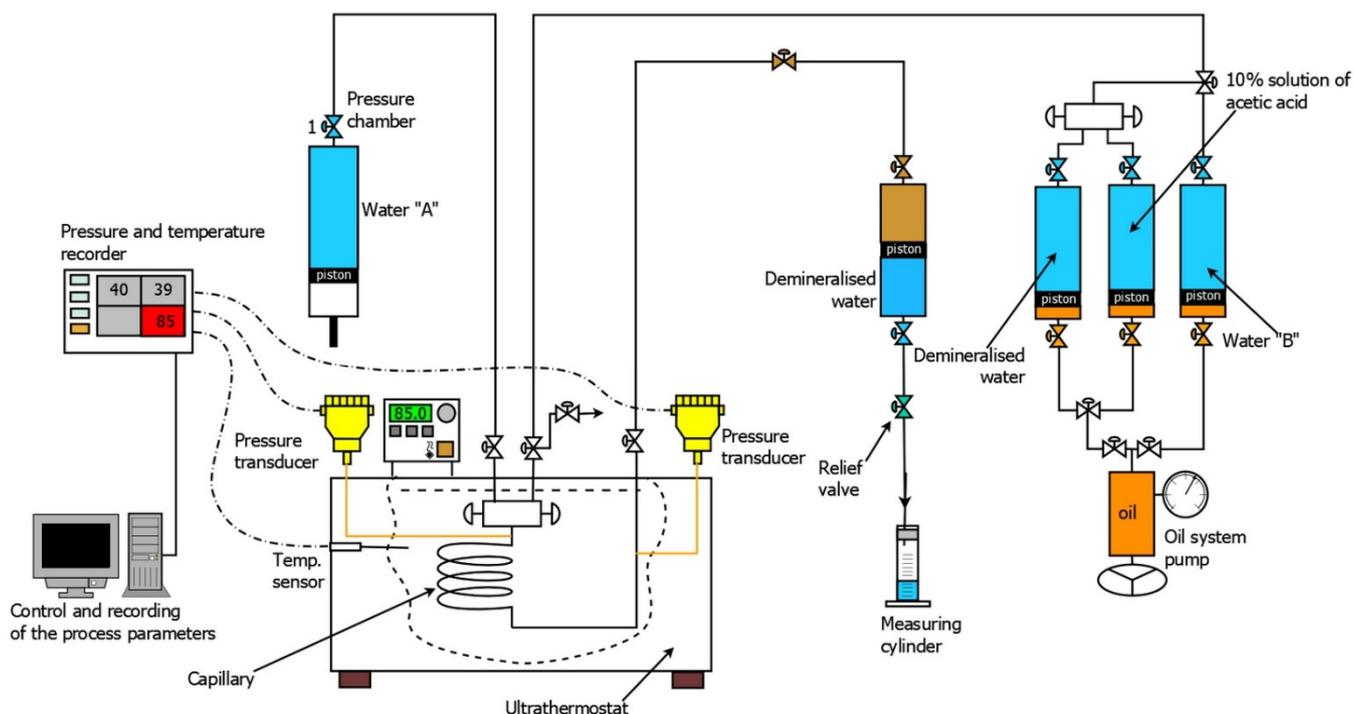
**Figure 1.** Measuring system diagram.
