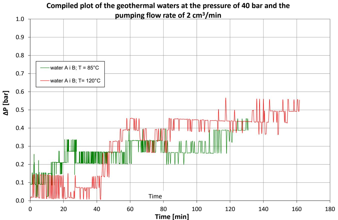
**Figure 3.** The course of the study of individual geothermal water types (measurement error is  $\pm 4\%$ ).
