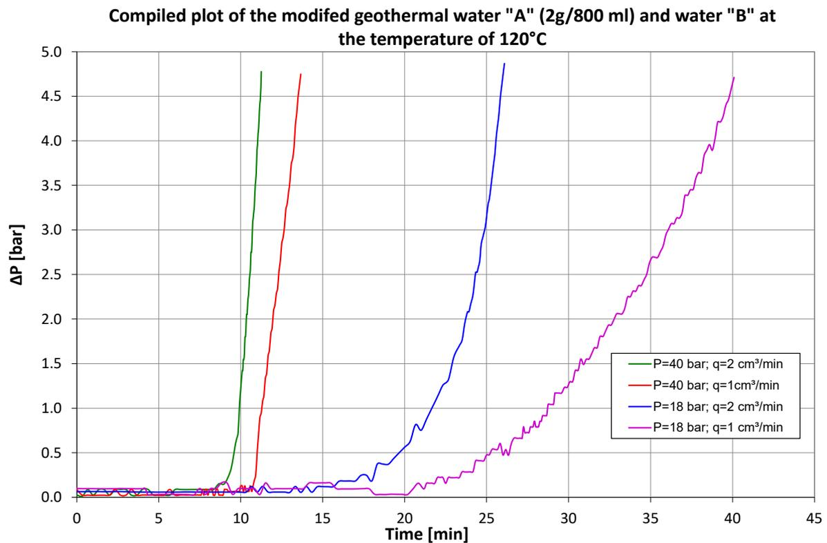
**Figure 5.** Tests for the precipitation of sediments for water “A” modified with sodium bicarbonate (2 g/800 mL) and water “B” at a temperature of 120 °C (measurement error is  $\pm 4\%$ ).
