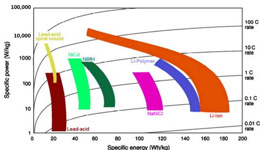
**Figure 8.** Distribution of different electrochemical batteries based on their energy densities and power [22,29].
