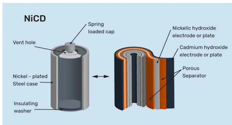
**Figure 12.** The nickel–cadmium battery’s fundamental structure [49].
