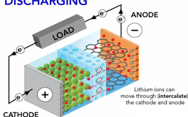
Figure 9. In-use lithium-ion battery operation [33].
