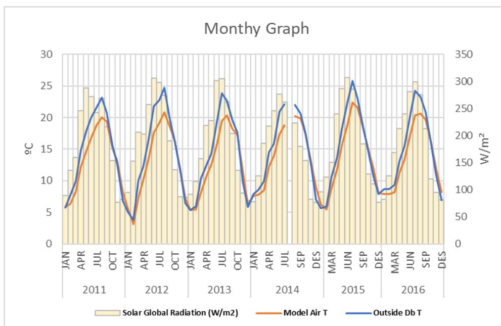
Figure 18. Comparison of outside and EnergyPlus model air temperatures.
