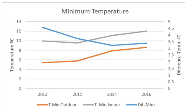
**Figure 17.** Minimum indoor and outdoor temperature and their difference in winter.
