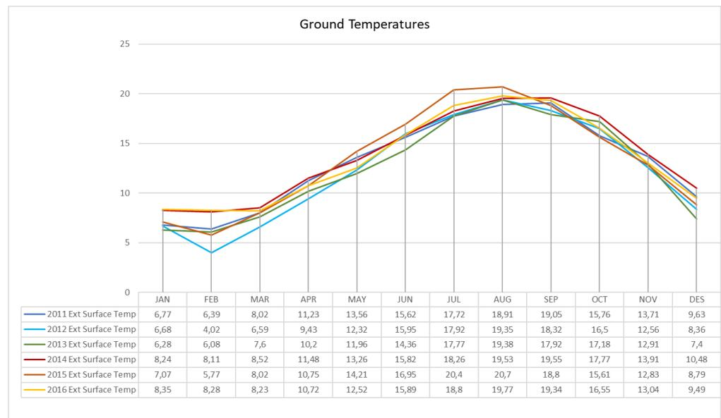
Figure 10. Ground temperatures.
