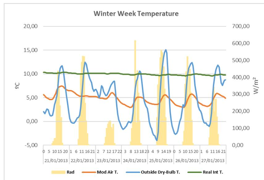
Figure 23. Hourly solar radiation, outdoor temperatures, and real and modeled indoor temperatures (winter).
