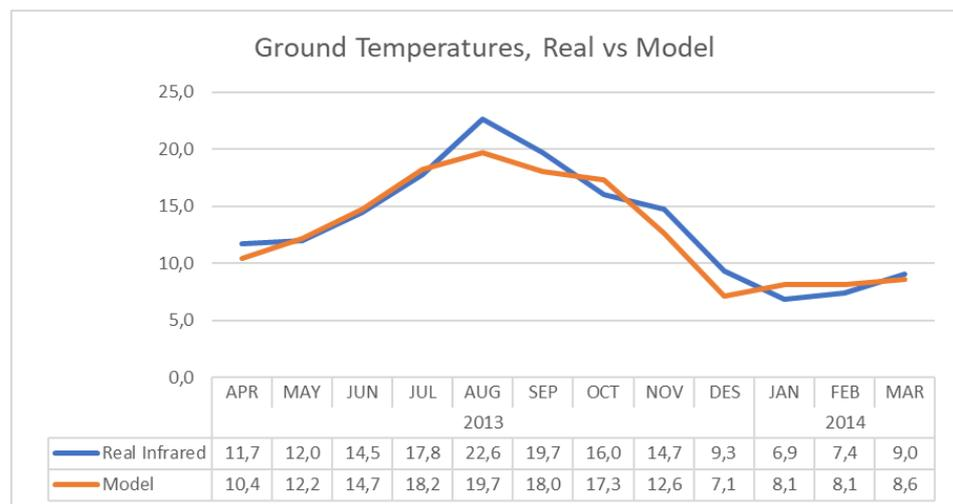
Figure 11. Ground temperatures, real vs. model.
