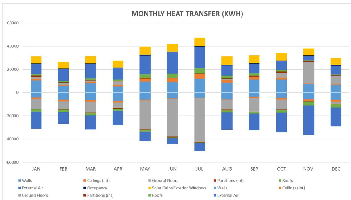
Figure 28. Monthly heat transfer in KWh.
