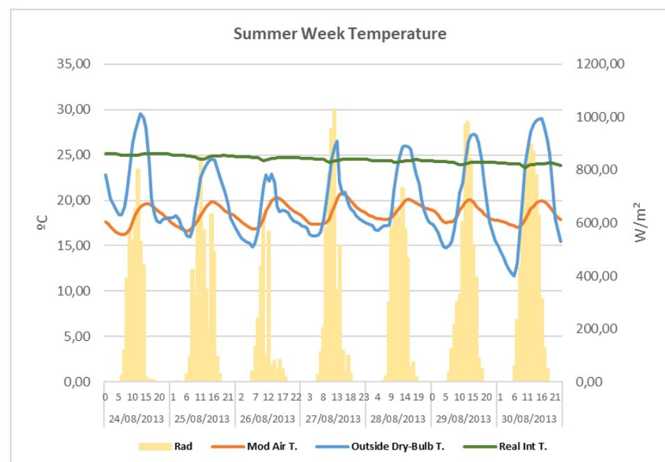
Figure 24. Hourly solar radiation, outdoor temperatures, and real and modeled indoor temperatures (summer).
