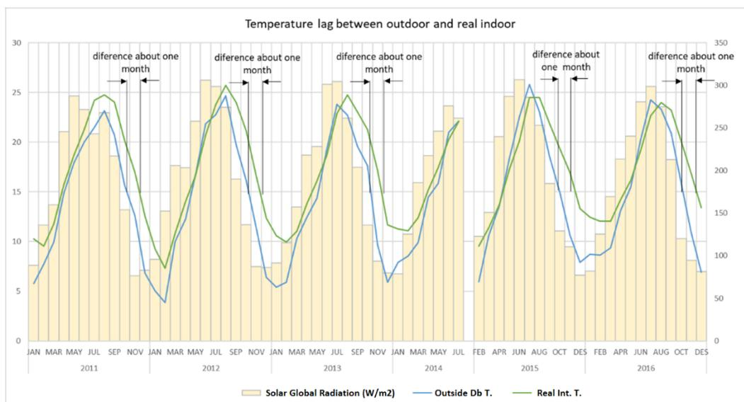
**Figure 15.** Comparison between average outdoor temperature and real average indoor temperature.
