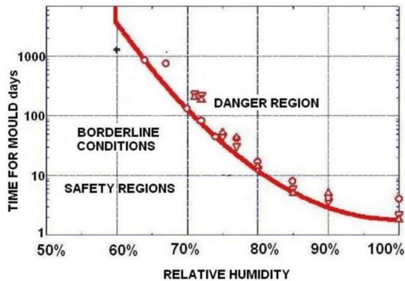
Figure 1. Time for mold formation according to relative humidity. Source: [23].
