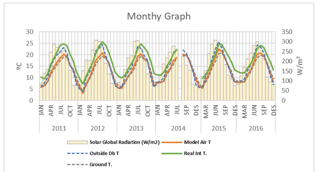
Figure 20. Comparison of real interior temperature and model temperature from the EnergyPlus model.
