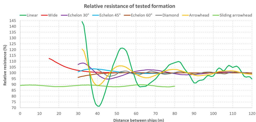
**Figure 15.** Relative value of total drag as a function of ship distance for a given formation in the entire speed range.
