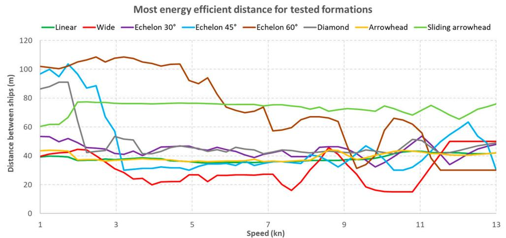
Figure 17. The distance that gives the least resistance for a given speed and shape of the formation.
