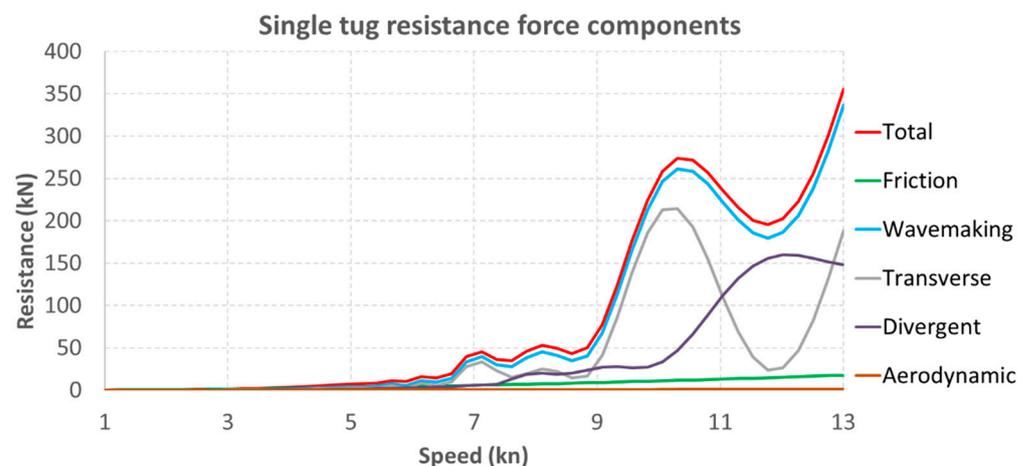
Figure 5. Resistance force components acting on a single tug used in a formation.
