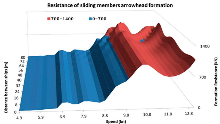
Figure 14. Total resistance of a formation composed of four tugboats sailing in a diamond-shaped formation.
