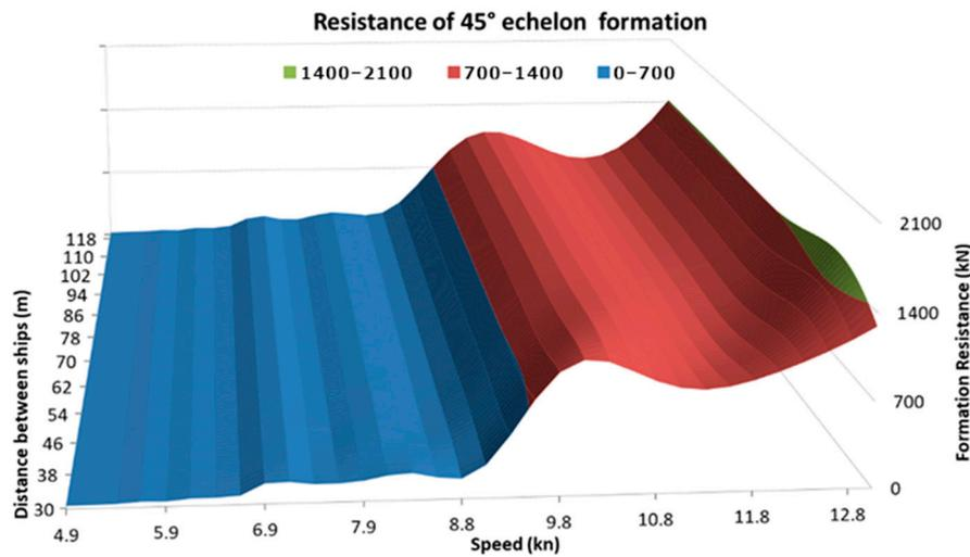
Figure 10. Total resistance of a formation consisting of four tugboats sailing in an echelon formation with an angle of 45°.
