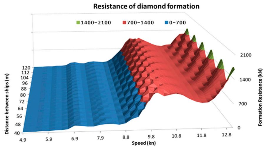
Figure 12. Total resistance of a formation composed of four tugboats sailing in a diamond-shaped formation.
