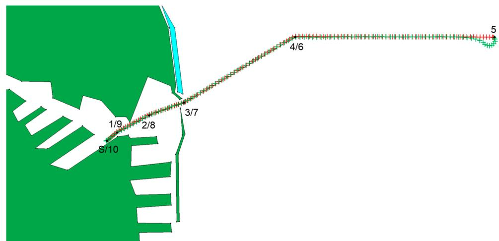
**Figure 19.** Route traveled by the simulated tugboat.
