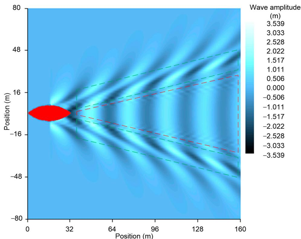
**Figure 4.** Waves forming behind the stern of a moving tugboat. Transverse waves marked with a red outline, divergent waves marked with a green outline.
