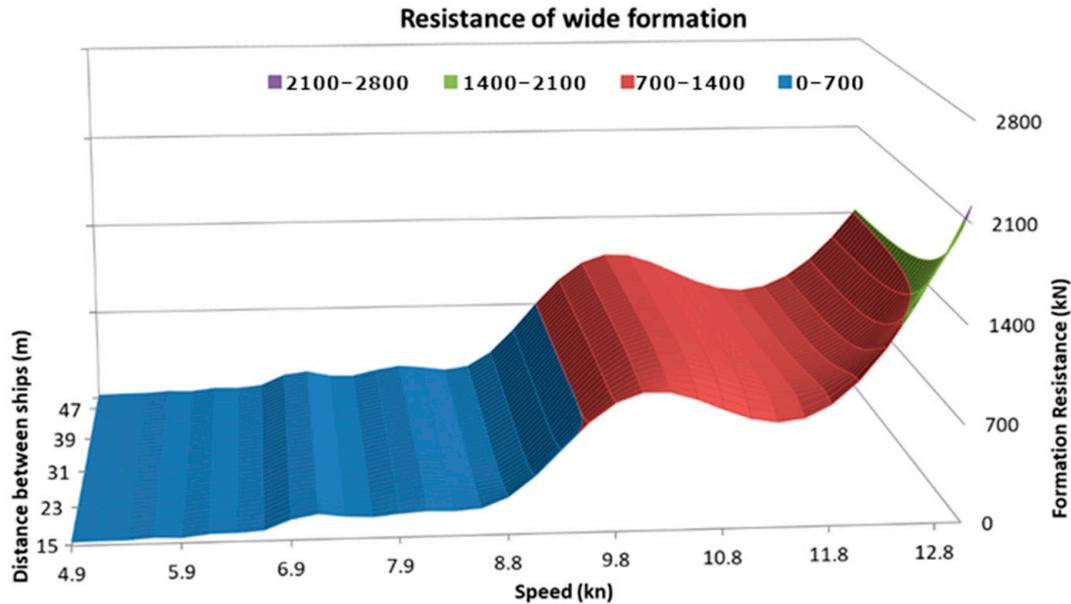
Figure 8. Total resistance of a formation composed of four tugboats sailing in wide formation.
