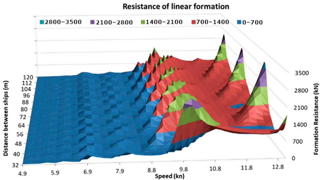
Figure 7. Total resistance of a formation composed of four tugboats sailing in a linear formation.
