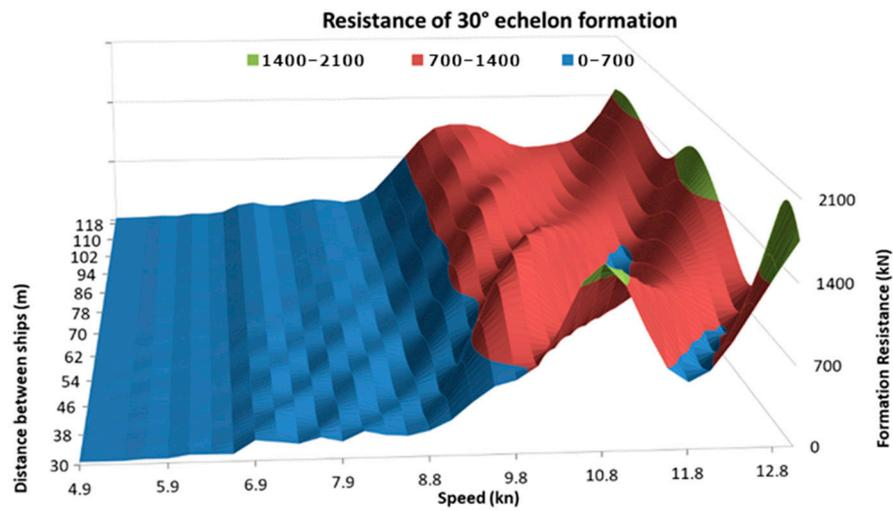
Figure 9. Total resistance of a formation consisting of four tugboats sailing in an echelon formation with an angle of 30°.
