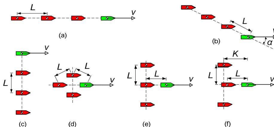
**Figure 6.** Considered formation shapes. (a) a linear shape, (b) an echelon shape with an angle of  $\alpha$ , (c) a wide shape, (d) diamond-shaped, (e) arrowhead-shaped, (f) arrowhead-shaped with variable position of outside members.
