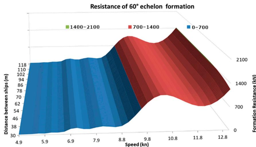
Figure 11. Total resistance of a formation consisting of four tugboats sailing in an echelon formation with an angle of 60°.
