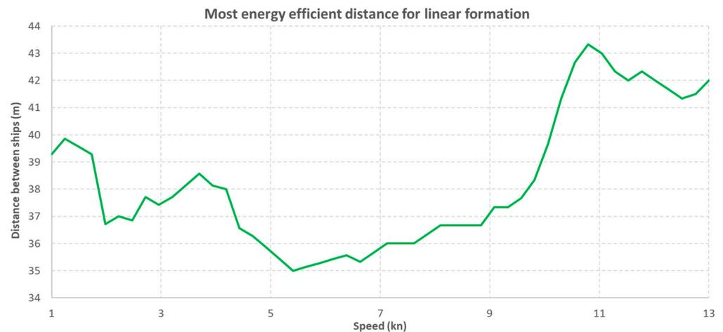
**Figure 18.** Distance providing the least resistance for a given formation speed in a linear formation.
