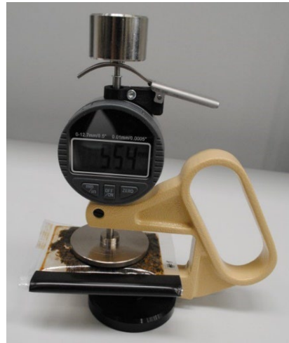
Figure 2. Checkline J-40-T digital gauge measuring the thickness of bee origin biological material samples.
