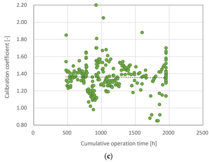
**Figure 3.** Calibration coefficient values according to cumulative operating time of cooling towers: (a) CT-1; (b) CT-2; (c) CT-3.
