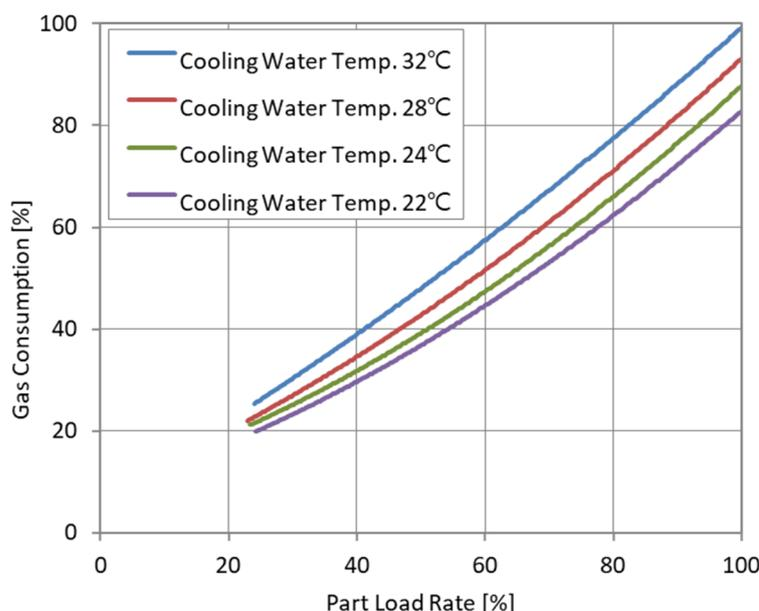
**Figure 1.** Performance curve of heat source equipment.
