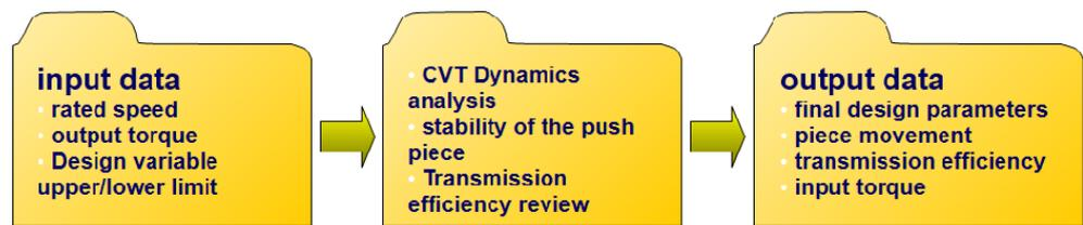
Figure 6. The principle of the design program for improving CVT performance.
