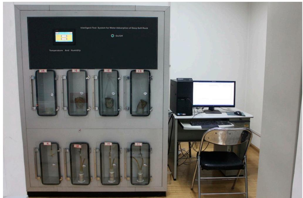
**Figure 1.** Physical experimental system for real-time experimental monitoring for water absorption evolution behaviors of sandstone in Mogao Grottoes, China.
