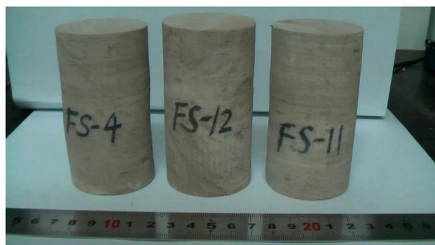
Figure 9. Sandstone samples used in this study reaches the saturation state at the end of the experiment.
