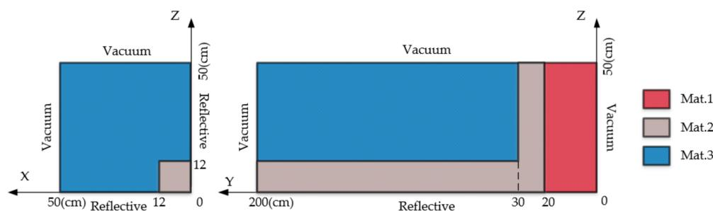
Figure 2. Geometry of the self-designed neutron streaming problem.
