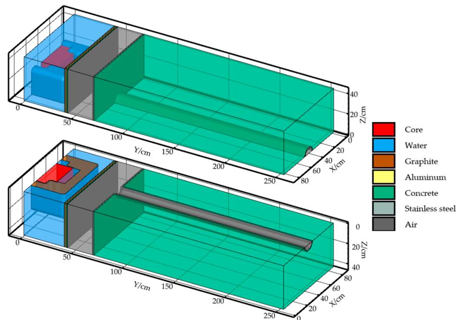
**Figure 8.** Geometry of the IRI-TUB benchmark problem.
