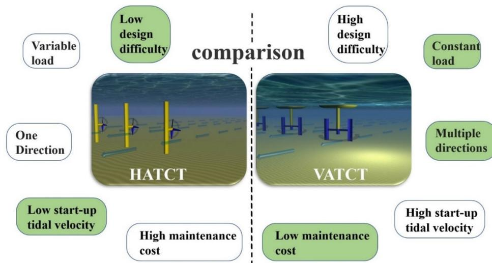
**Figure 11.** The comparison of HATCT and VATCT.
