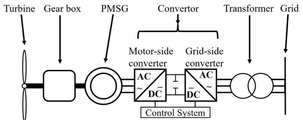
Figure 9. PMSG-based tidal TCG system.
