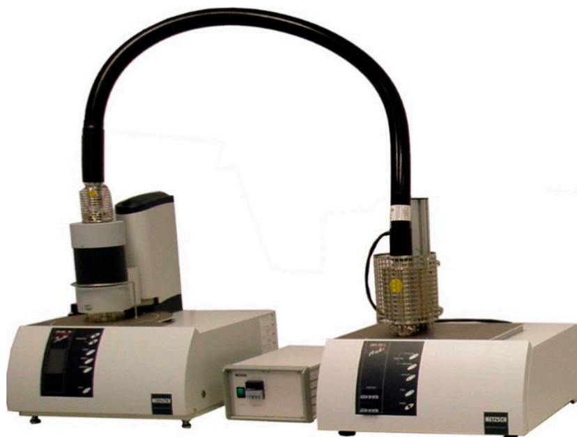
Figure 5. Analyzer NETZSCH STA 449 Jupiter F1 coupled with QMS Aëolos analyzer.
