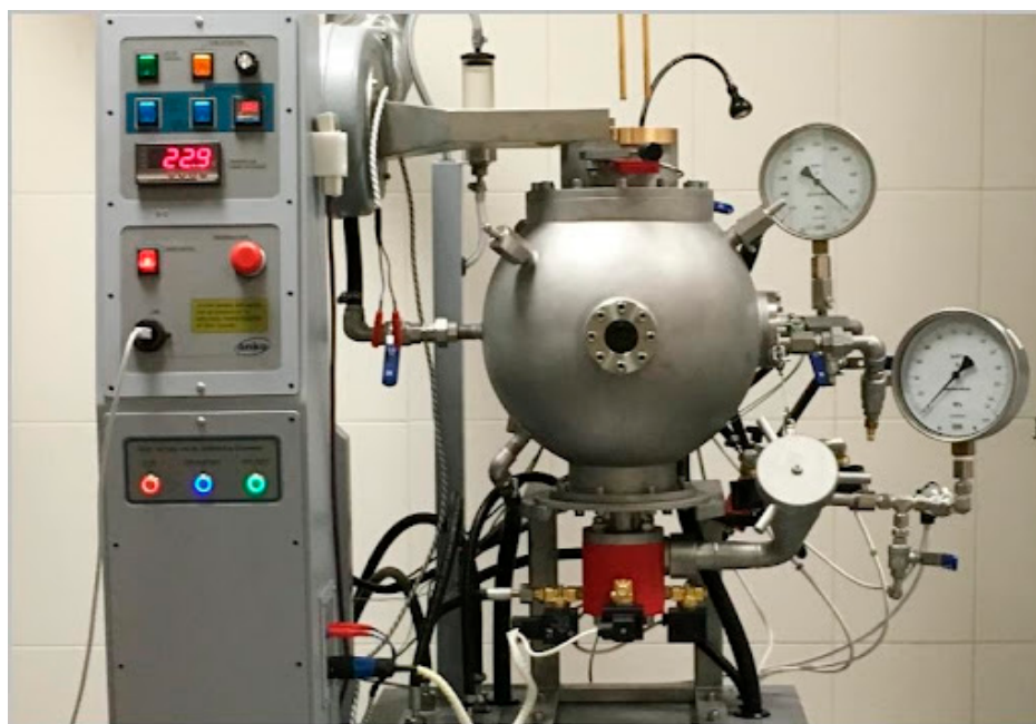
Figure 6. Twenty-liter spherical vessel manufactured by ANKO S.A.
