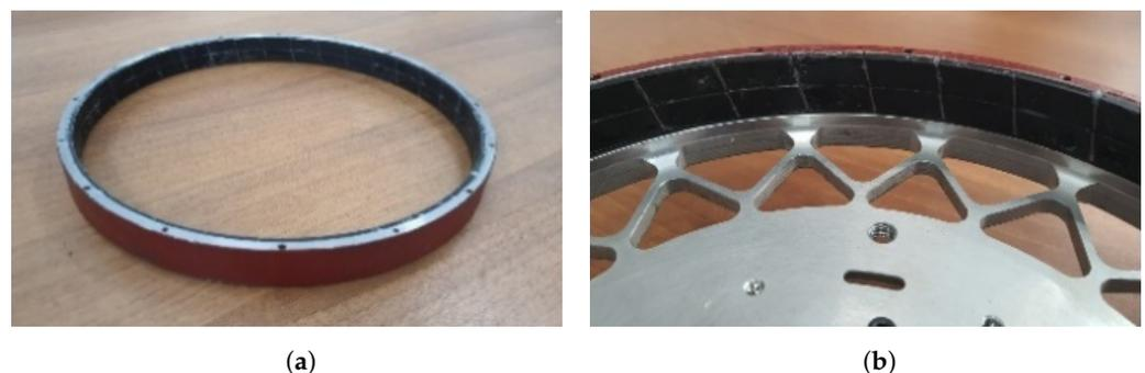
**Figure 22.** (a) Rotor structure. (b) Magnet segmentation.
