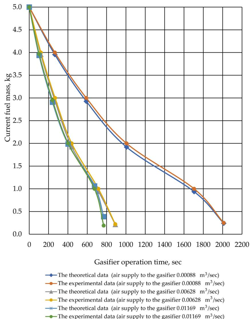
**Figure 2.** Comparison of the experimental and theoretical indicators of the change of fuel mass when using wood pellets.
