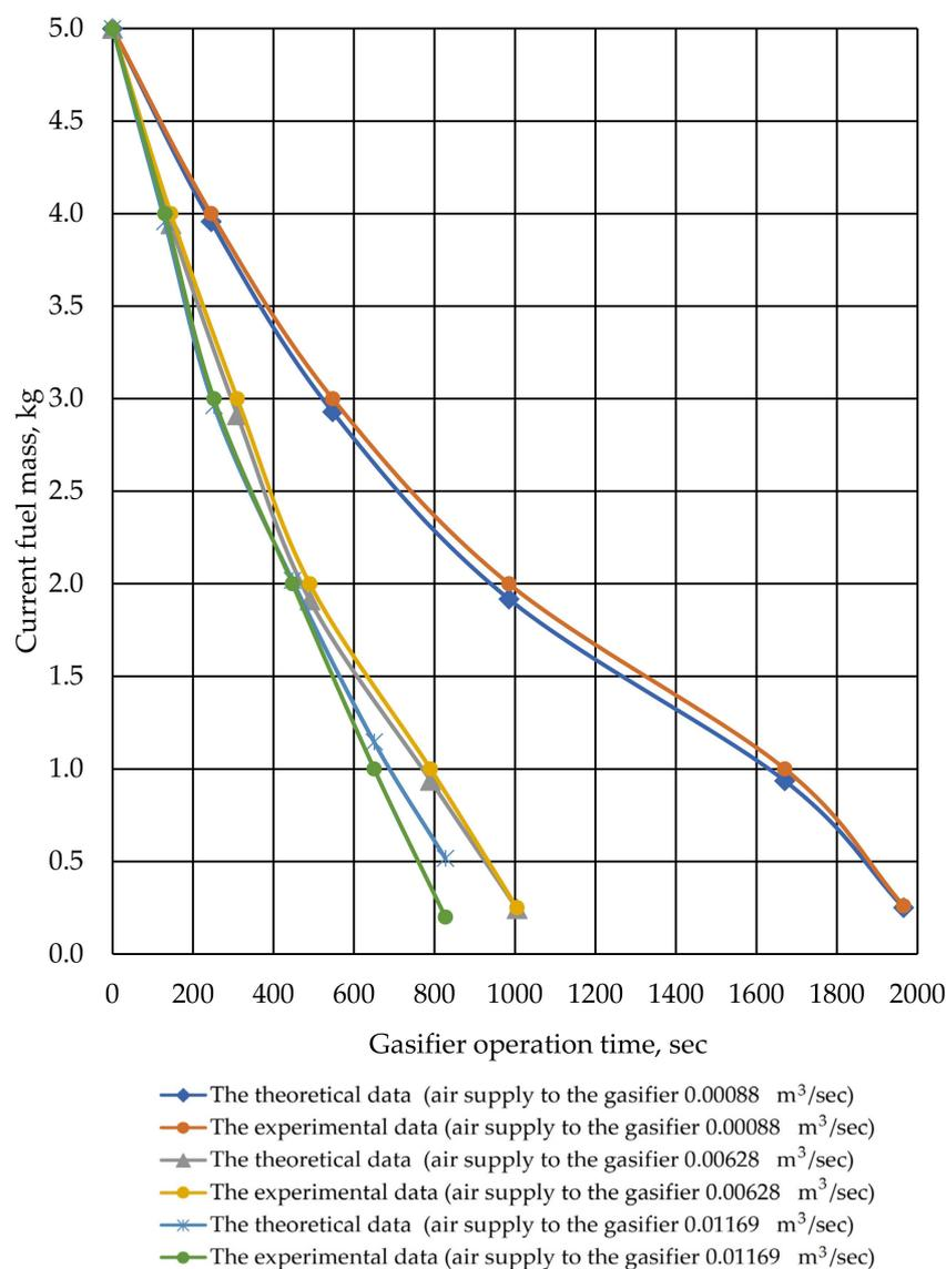
**Figure 3.** Comparison of the experimental and theoretical indicators of a change of fuel mass when using straw pellets.
