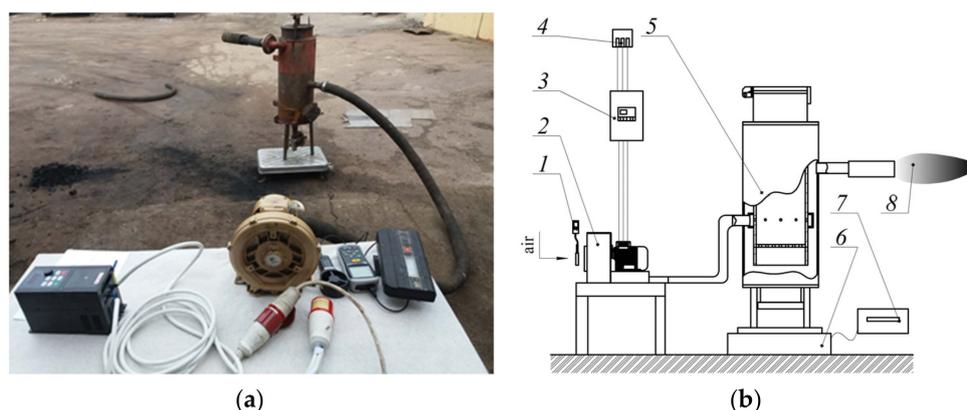
**Figure 1.** General view (a) and schematic diagram (b) of an experimental facility: 1—anemometer Tenmars TM-402; 2—blower Goorui GHBH-0D5-34-1R2; 3—frequency converter Hitachi-3G3JX-A4075-EF; 4—power supply 0.4 kW; 5—downdraft gasifier; 6—scales; 7—scales indicator; 8—generator gas torch.
