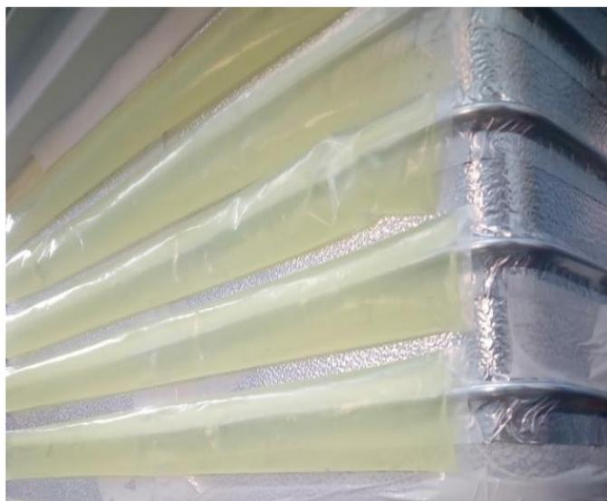
**Figure 9.** Application of a gelatinized eutectic PCM to the evaporator of a prototype chest freezer (photo courtesy: Vítor Silva, Tensai Indústria S.A., Portugal).
