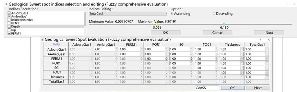
Figure 5. Schematic diagram of parameter selection, sectional interval setting and parameter weight design (in-house development software platform interface).
