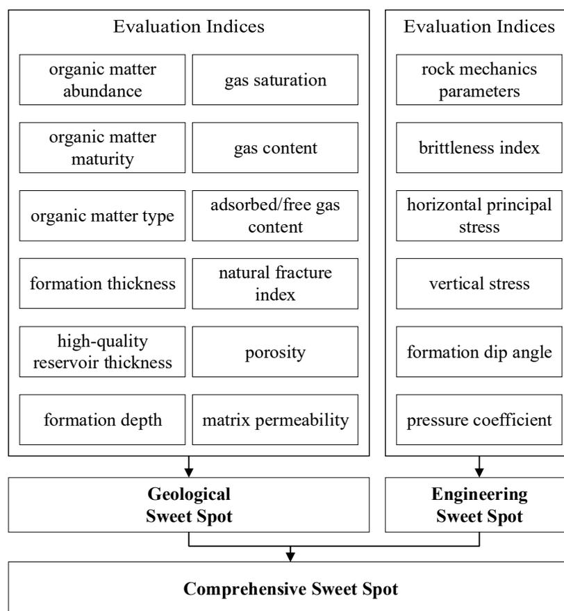
**Figure 1.** Evaluation index system and evaluation indices of shale gas sweet spots.
