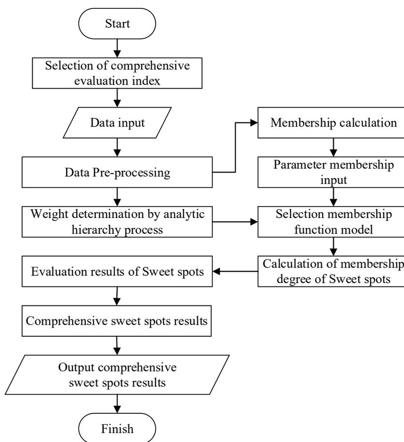
**Figure 3.** Technical process of comprehensive sweet spots using fuzzy comprehensive evaluation directly based on evaluation parameters.
