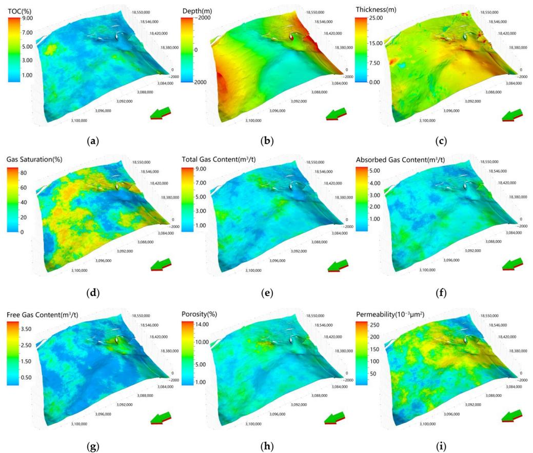
Figure 6. Three-dimensional evaluation index model of geological sweet spots in the study area: (a) organic matter abundance (TOC); (b) reservoir formation thickness; (c) reservoir burial depth; (d) gas saturation; (e) total gas content; (f) adsorbed gas content; (g) free gas content; (h) porosity; (i) matrix permeability (models visualized by Schlumberger Petrel software).
