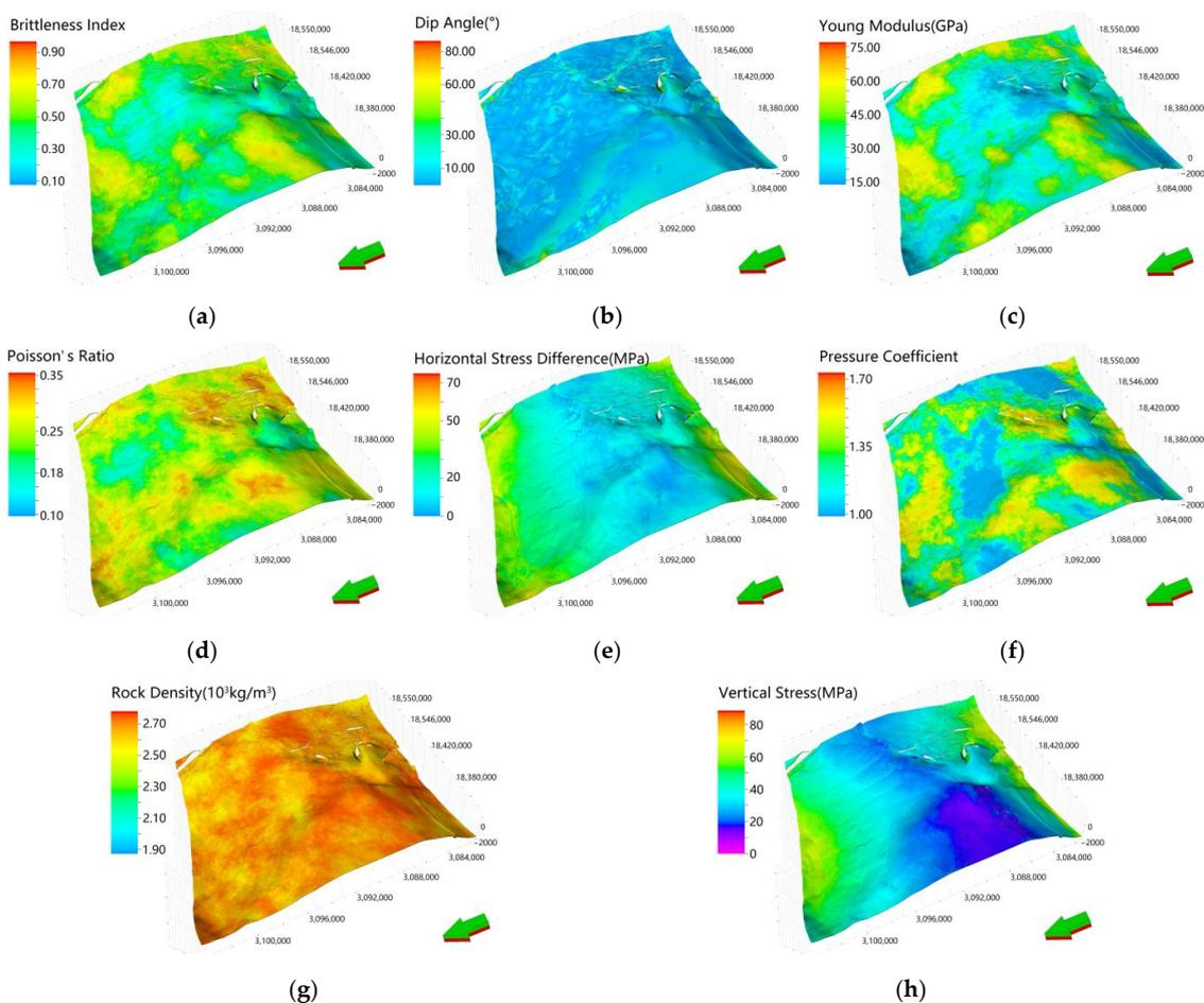
**Figure 7.** Three-dimensional evaluation index model of engineering sweet spots in the study area: (a) brittleness index; (b) formation dip angle; (c) Young modulus; (d) Poisson's ratio; (e) horizontal stress difference; (f) pressure coefficient; (g) rock density; (h) vertical stress (models visualized by Schlumberger Petrel software).
