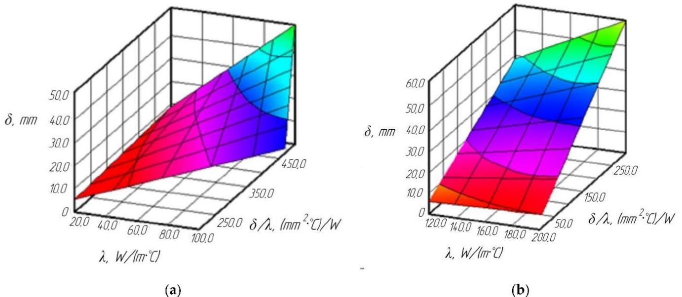
**Figure 4.** Changes in thermal resistance ( $\delta/\lambda$ ) of brake discs depending on their thickness ( $\delta$ ) and thermal conductivity coefficients of the materials ( $\lambda$ ), varying within: (a) 20–100  $\text{W}/(\text{m}^2 \cdot \text{C})$ ; (b) 120–200  $\text{W}/(\text{m}^2 \cdot \text{C})$ .
