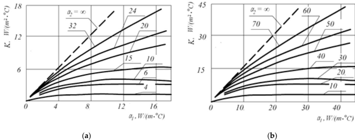
**Figure 6.** Change in the heat transfer coefficient  $K$  depends on the heat transfer coefficient from the outer  $\alpha_1$  and inner  $\alpha_2$  surfaces of the left half-disc self-ventilated brake disc of a MAN truck model TGA 26.430 when driving at a speed of: (a) 30 km/h; (b) 60 km/h [24].
