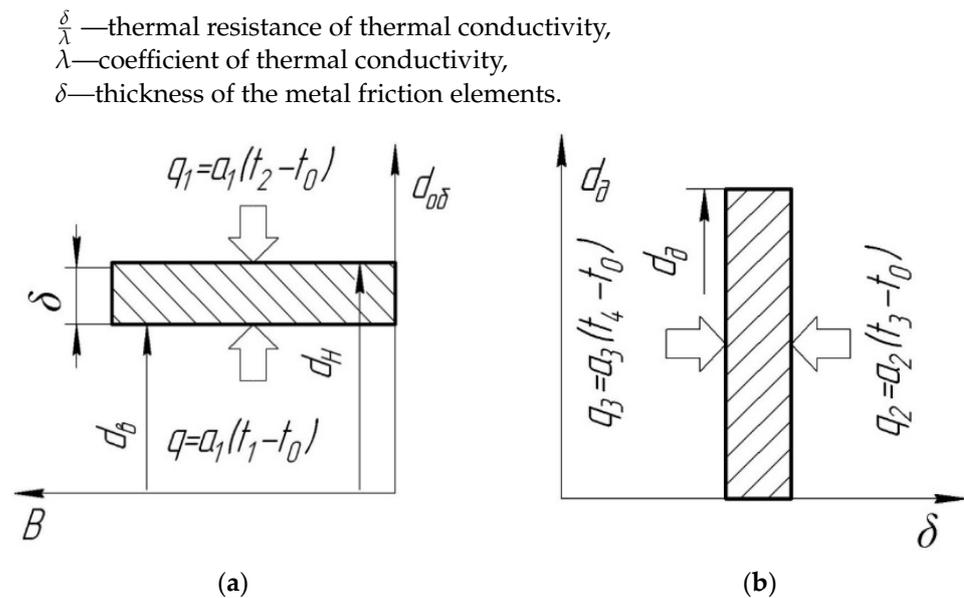
**Figure 2.** Design parameters of metal friction elements: (a) working surfaces of the pulley rim and drum; (b) surfaces of a solid-disc and heat fluxes generated on their working surfaces. In figure:  $d_b$ ,  $d_H$ ,  $d_a$ —diameters: inner drum; outer pulley; solid disc;  $B$ ,  $\delta$ —width and thickness of elements;  $q_i$ —heat fluxes;  $t_i$ —surface temperatures;  $t_0$  is the ambient temperature.
