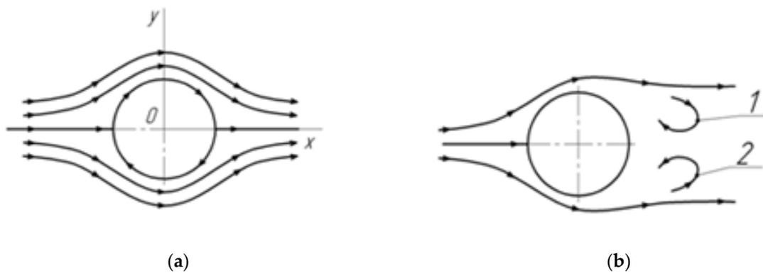
**Figure 3.** Air flow around the non-working and working surfaces of the drum and pulley rim: (a) non-circulating; (b) circulating; 1, 2—inside different directions [25].
