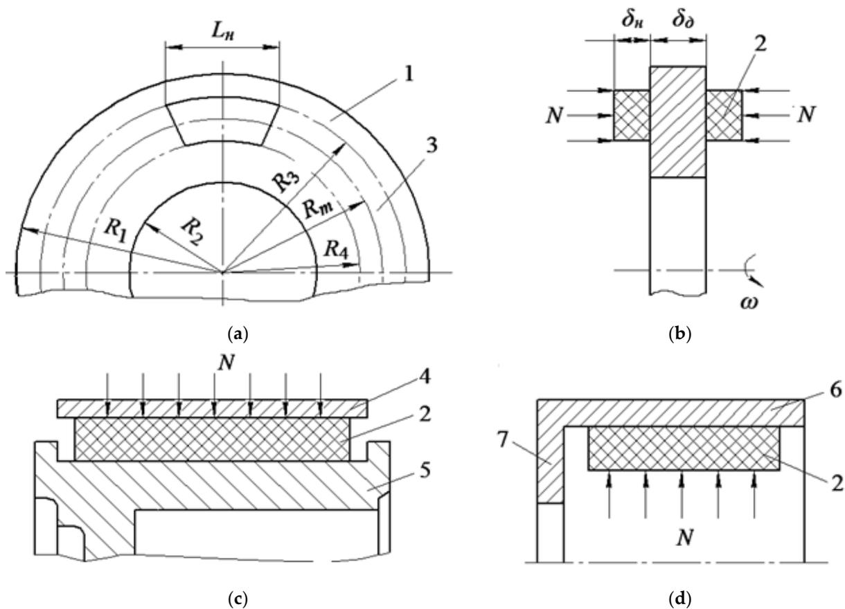
**Figure 1.** Diagrams of the different types of friction units of braking devices: (a) longitudinal section of disc-shoe; (b) transverse section disc-shoe; (c) cross-section of tape-shoe; (d) cross-section drum-shoe.
