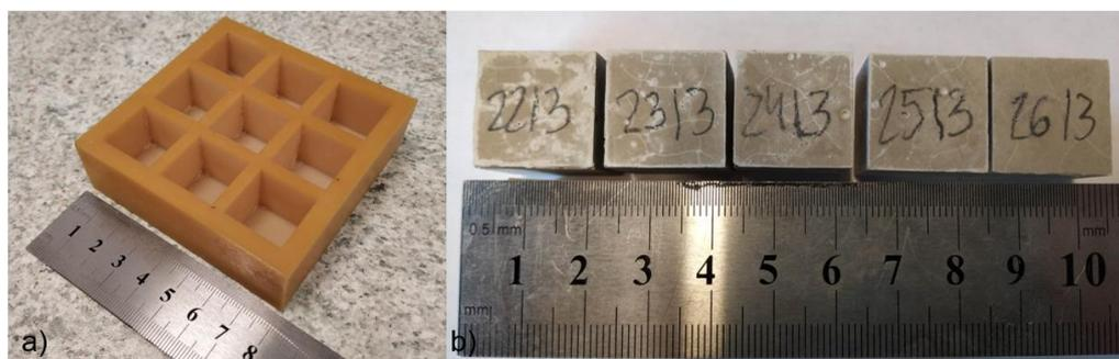
**Figure 2.** (a) Polyurethane mould; (b) cracking of the binder specimens after curing in water.
