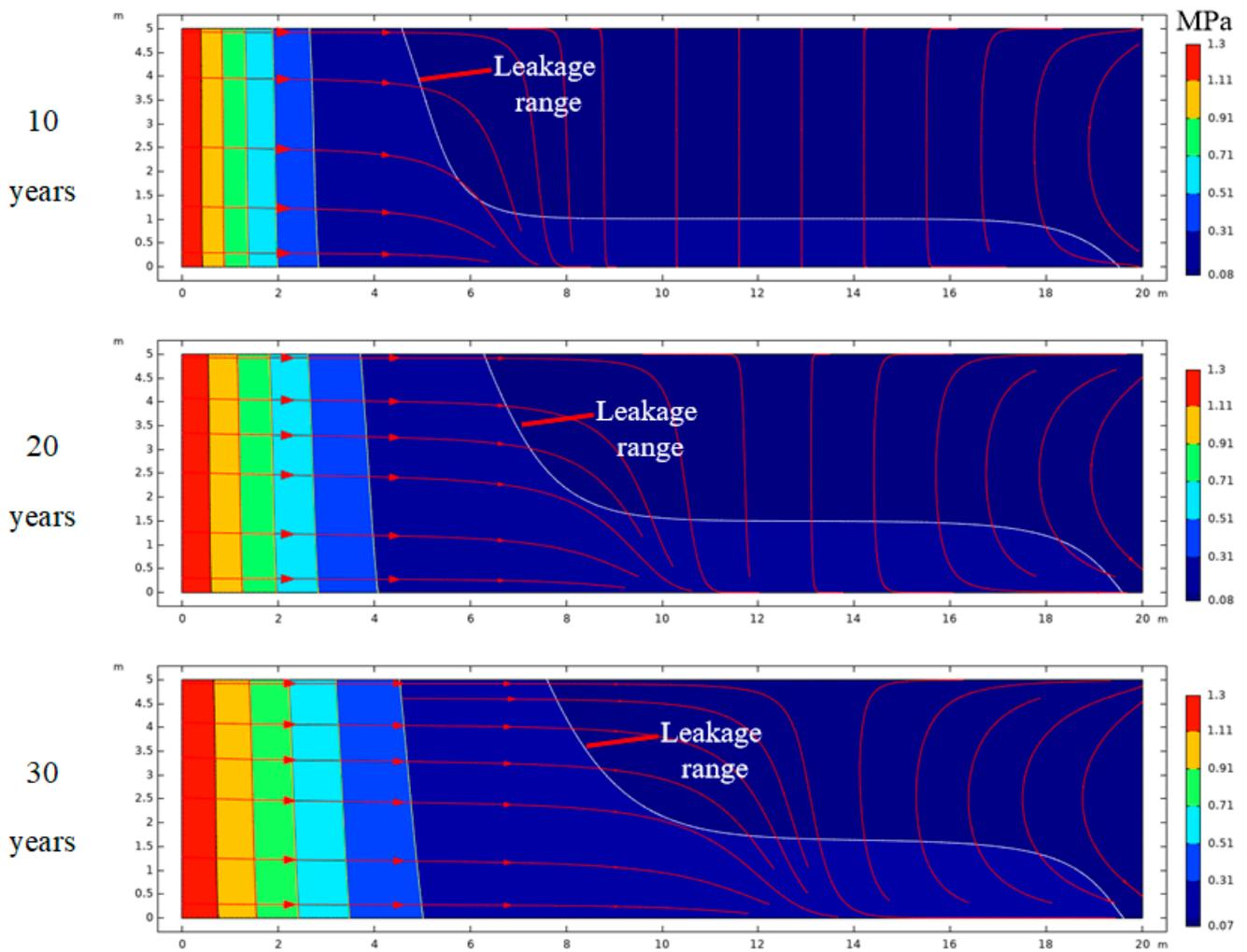
Figure 2. Evolution of leakage range in the coal pillar dam with the depth of 100 m (Unit: MPa).
