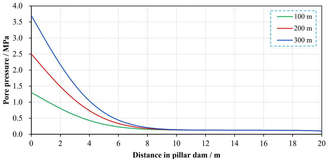
**Figure 6.** Comparison of pore pressure in the coal pillar dam body under different depths.
