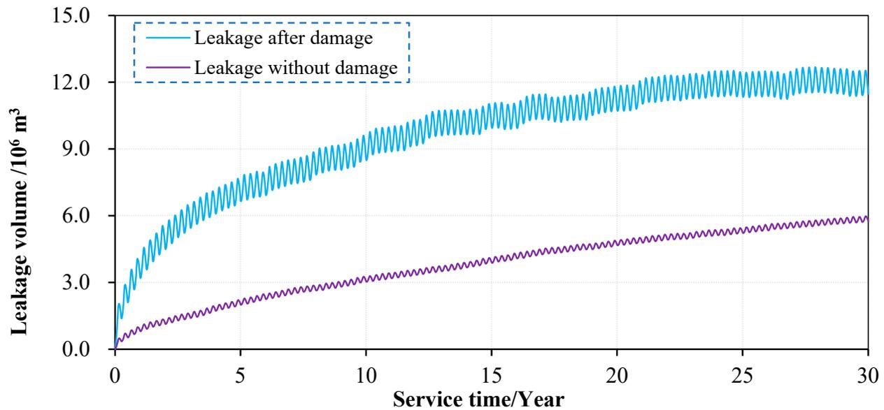
**Figure 16.** Comparison of cumulative leakage volume between the damaged and undamaged coal pillar dam.
