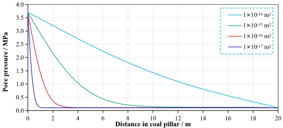
Figure 11. Pore pressure distribution of the coal pillar dam under different permeability.
