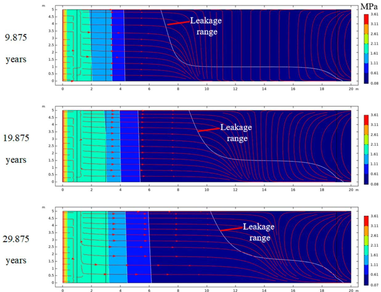
**Figure 14.** Changes of leakage range with time.
