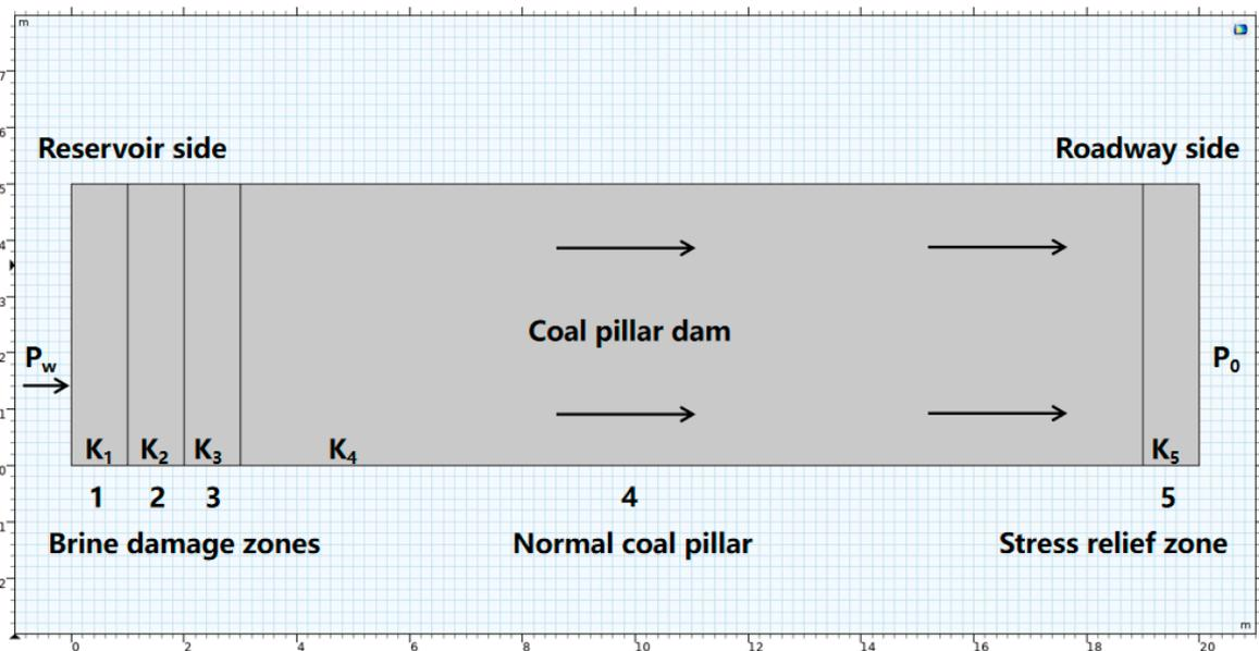
Figure 13. Schematic diagram of damage zone distribution in the coal pillar dam.
