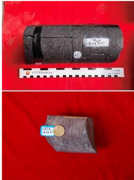
Figure 2. Core samples of shale.
