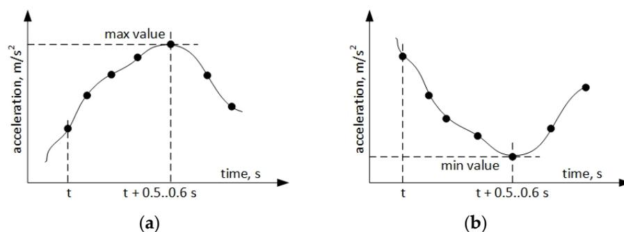
**Figure 5.** Diagrams of the method adopted to identify maneuvers and their extreme values: (a) acceleration, (b) braking.
