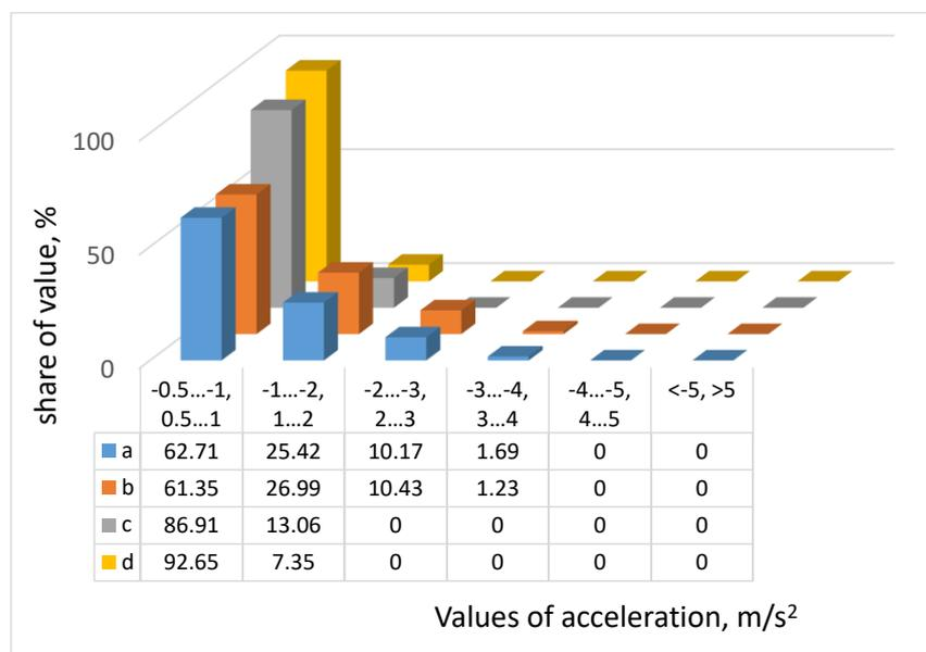
**Figure 10.** Distributions of absolute values of the extreme of lateral acceleration during turning maneuvers for various route sections: (a) city road; (b) suburban road; (c) expressway (dual carriageway); (d) highway.
