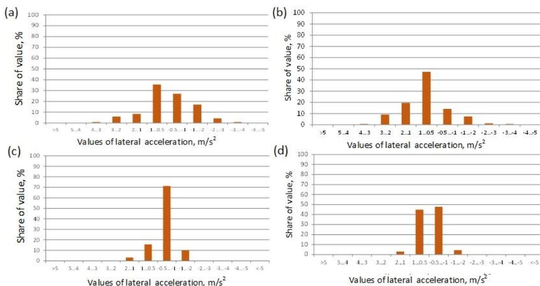
**Figure 9.** Distributions of the extreme values of lateral acceleration during turning maneuvers for various route sections; route sections: (a) city road; (b) suburban road; (c) expressway (dual carriageway); (d) highway.
