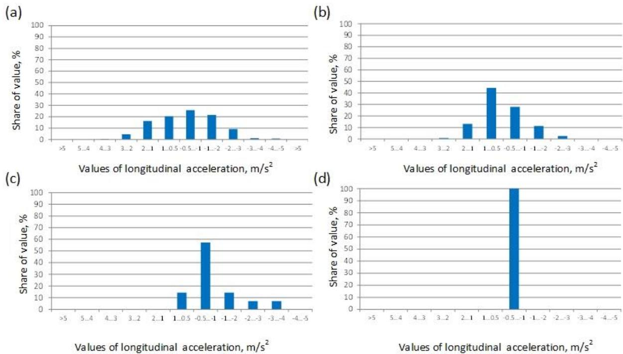
**Figure 8.** Distribution of the extreme values of longitudinal acceleration and deceleration maneuvers for various route sections: (a) city road; (b) suburban road; (c) expressway (dual carriageway); (d) highway.
