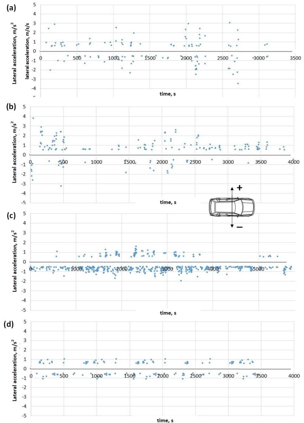
**Figure 7.** Lateral acceleration extreme values in the right and left turning maneuvers on the different sections of the route: (a) city road; (b) suburban road; (c) expressway (dual carriageway); (d) highway.
