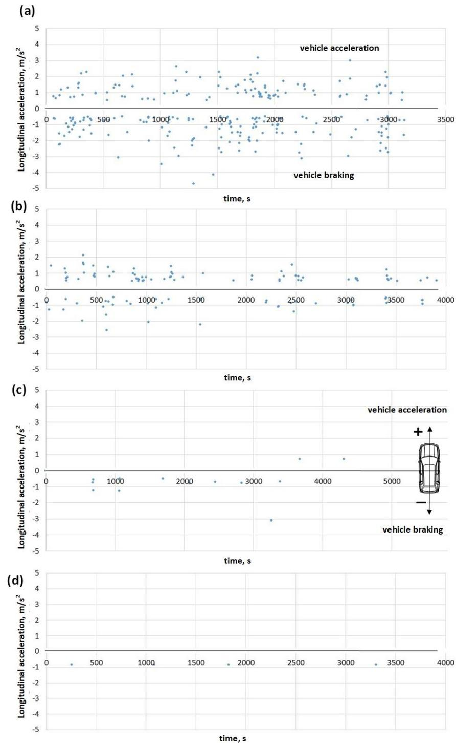
**Figure 6.** Longitudinal acceleration extreme values in the acceleration and braking maneuvers in the various sections of the route: (a) city road; (b) suburban road; (c) expressway (dual carriageway); (d) highway.
