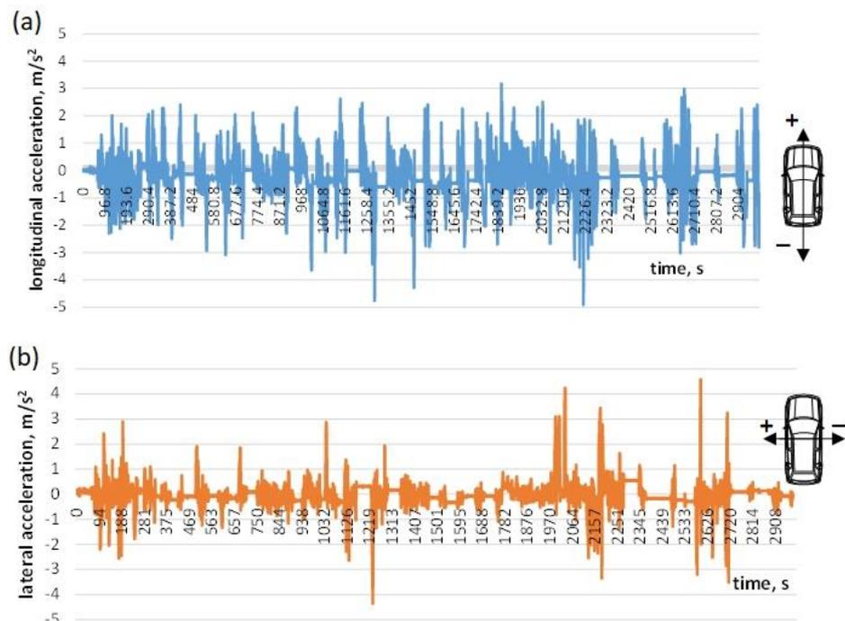
Figure 4. The examples of recorded values of the vehicle acceleration: (a) longitudinal; (b) lateral.
