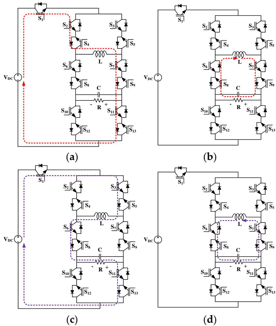
**Figure 3.** Equivalent circuits of UPC for different modes of operation during DC–AC conversion (inverter operation): (a) Mode-1, (b) Mode-2, (c) Mode-3, (d) and Mode-4.
