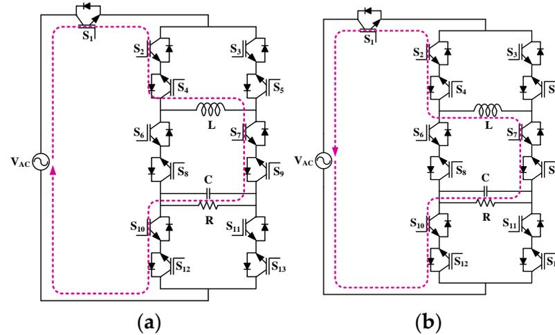
**Figure 5.** Equivalent circuits of different modes operation during AC voltage controller operation: (a) Mode-1 and (b) Mode-2.
