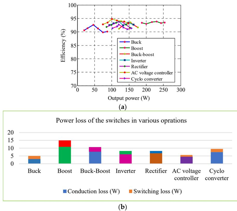
**Figure 14.** (a) The proposed converter efficiency in the different operation modes and (b) power loss of the switches in various operations.
