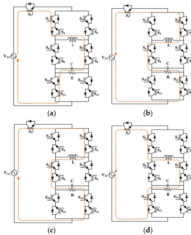
**Figure 7.** Equivalent circuits of different modes operation during cyclo-converter operation: (a) Mode-1, (b) Mode-2, (c) Mode-3, and (d) Mode-4.
