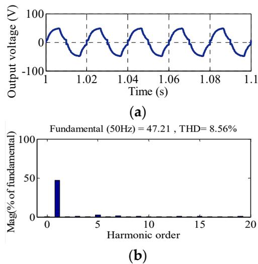
**Figure 9.** Simulation results of proposed UPC in inverter mode: (a) inverter output voltage and (b) FFT analysis.
