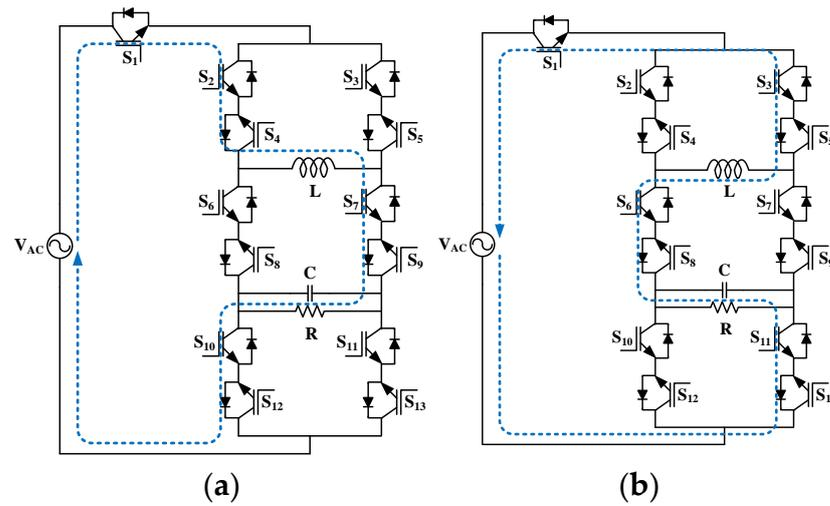
**Figure 4.** Equivalent circuits of different modes operation during rectifier operation: (a) Mode-1 and (b) Mode-2.
