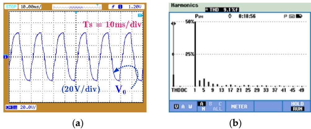
Figure 12. Experimental results of UPC in inverter operation: (a) output voltage and (b) FFT analysis.
