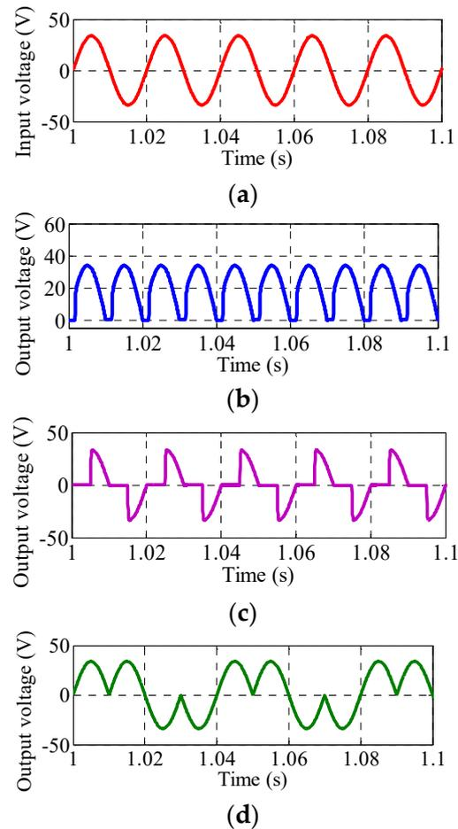
**Figure 10.** Simulation results of the proposed UPC in rectifier, AC voltage controller, and cyclo-converter mode: (a) input voltage, (b) rectifier output voltage, (c) AC voltage regulator output voltage, and (d) cyclo-converter output voltage.
