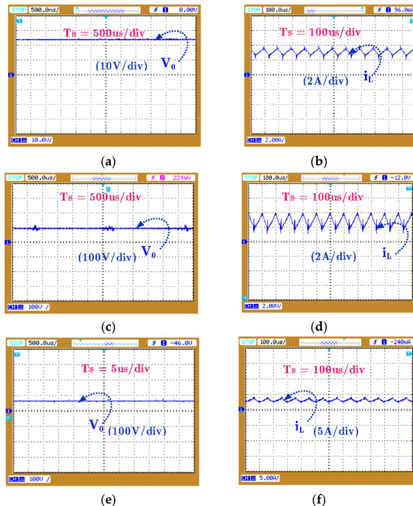
**Figure 11.** Experimental results of proposed UPC in DC–DC operation: (a) buck output voltage, (b) inductor current in buck operation, (c) boost output voltage, (d) inductor current in boost operation, (e) buck–boost output voltage, and (f) inductor current in buck–boost mode of operation.
