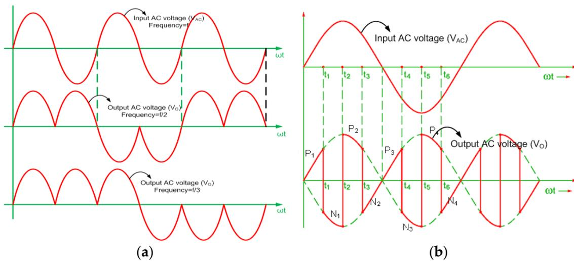
**Figure 6.** (a) Cyclo-converter’s typical output voltage waveform for step-down operation and (b) cyclo-converter’s typical output voltage waveform for step-up operation ( $f_o = 2f$ ).
