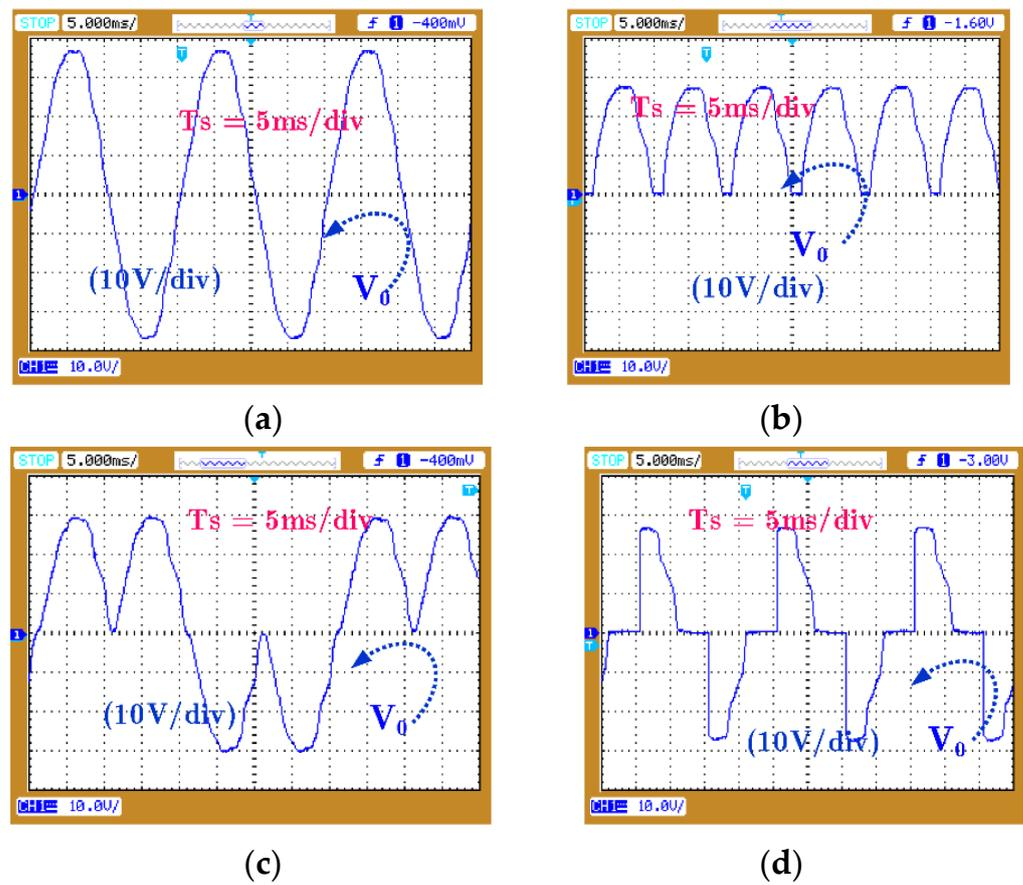
Figure 13. Experimental results of the proposed UPC in rectifier, AC voltage controller, and cyclo-converter mode: (a) input voltage, (b) rectifier output voltage, (c) AC voltage regulator output voltage, and (d) cyclo-converter output voltage.
