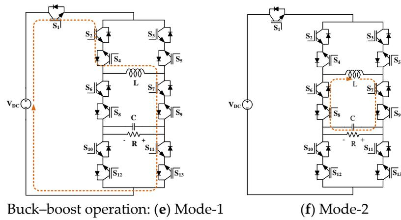
**Figure 2.** Equivalent circuits of UPC during DC–DC conversion: buck mode (a,b), boost mode (c,d), and buck–boost mode (e,f) of operation.
