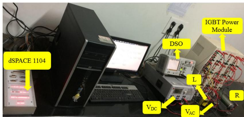
**Figure 15.** Snapshot of the hardware experimentation on the UPC prototype circuit in the laboratory.
