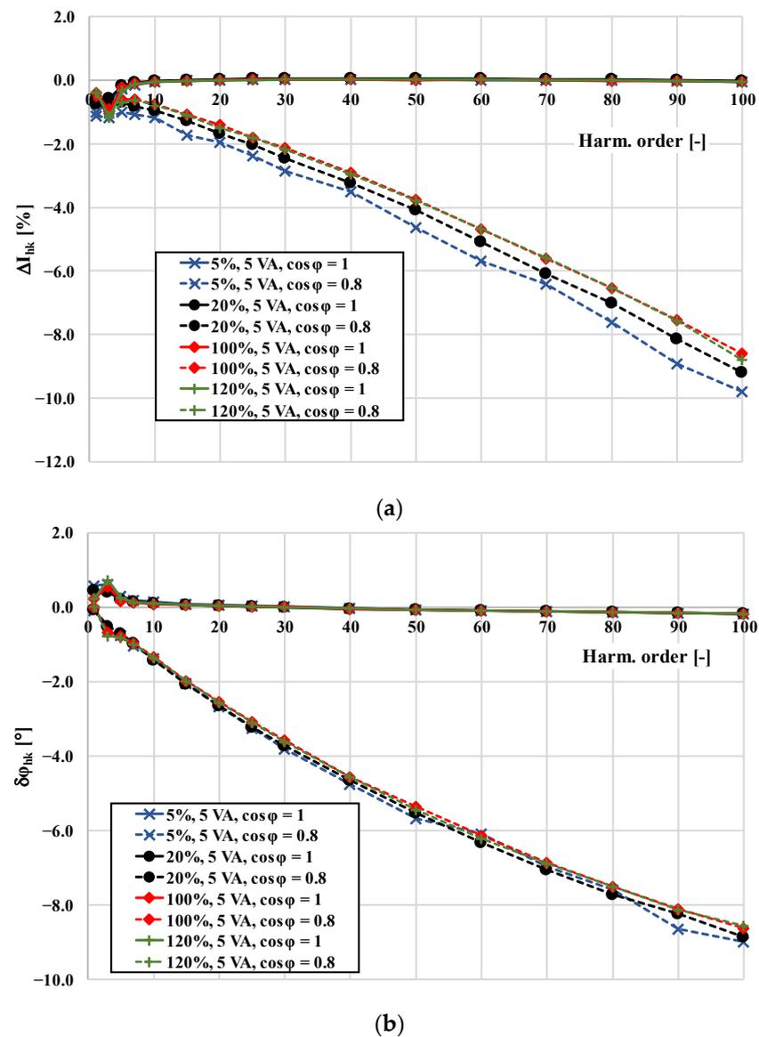
**Figure 4.** Comparison of the influence of the secondary winding rated load with power factor 0.8 inductive and 1.0 of a 300 A/5 A CT on: (a) current error; (b) phase displacement.
