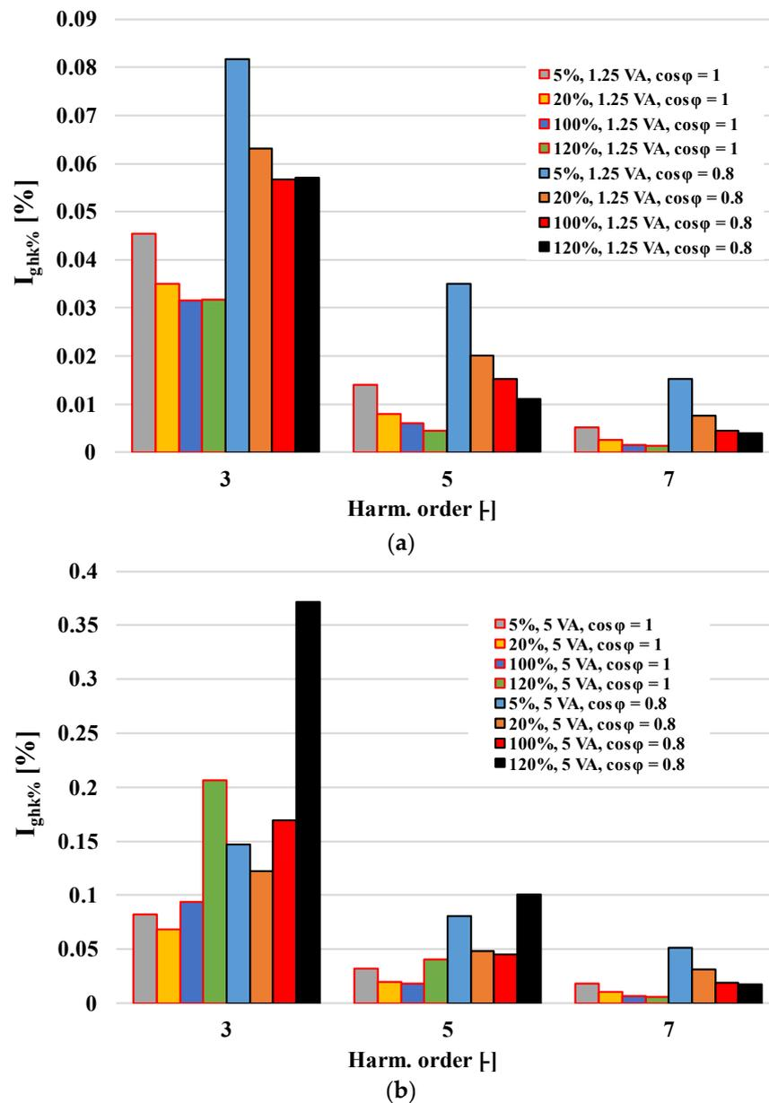
**Figure 6.** The levels of the generated harmonics in the secondary current by the inductive CT determined for 25% of the rated load (a) and for a rated load (b) with the power factors 0.8 inductive and 1.0.
