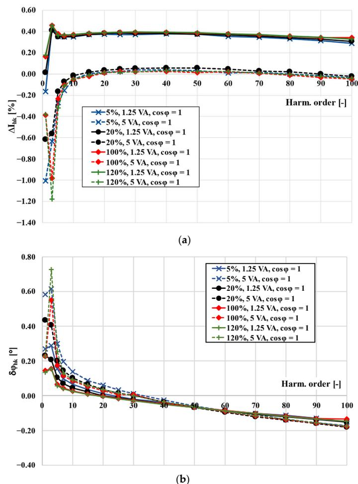
**Figure 2.** Influence of the secondary winding resistive load of a 300 A/5 A CT on its transformation accuracy: (a) current error; (b) phase displacement.
