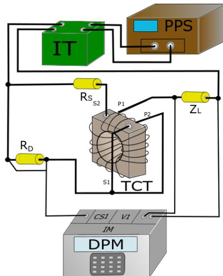
**Figure 1.** Measuring setup used for evaluation of values of current error and phase displacement of the CTs.
