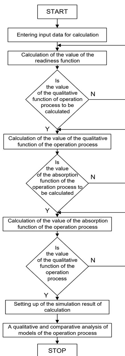
**Figure 2.** Algorithm of simulation studies on the quality of the evaluation of the exploitation process of a technical object.
