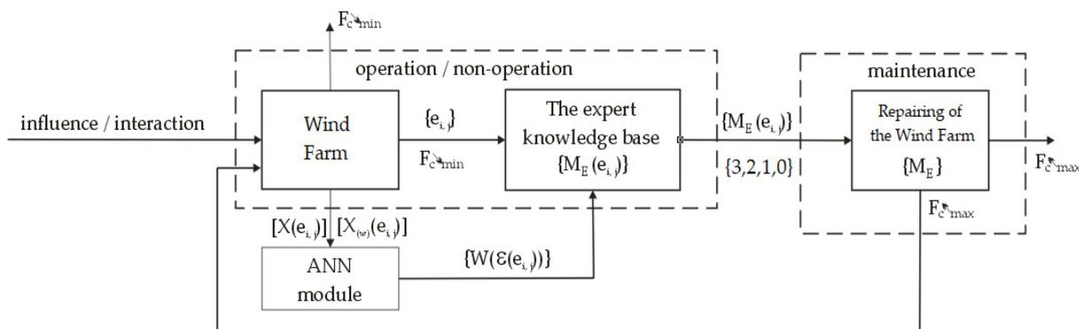
**Figure 1.** A schematic of the process of exploitation of a technical object using an artificial neural network.
