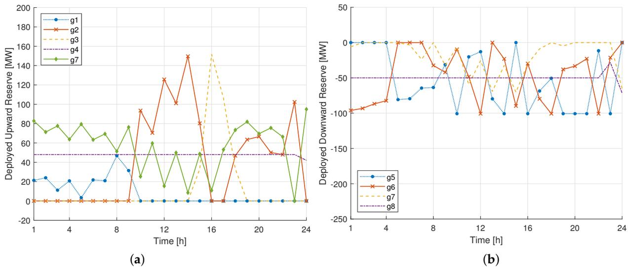
**Figure 7.** Optimal reserve deployments when reserves are considered in the ramp constraint: (a) upward operating reserve; (b) downward operating reserve.
