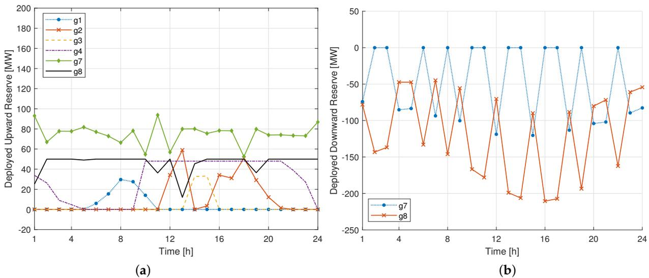
**Figure 6.** Optimal reserve deployments when the feasibility constraints are not implemented. (a) Upward operating reserve; (b) Downward operating reserve.
