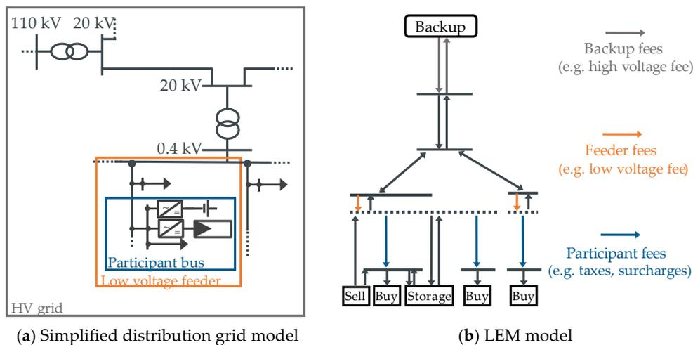
**Figure 2.** Modeling simplification of distribution grid topology (a) within the LEM market matching model (b).
