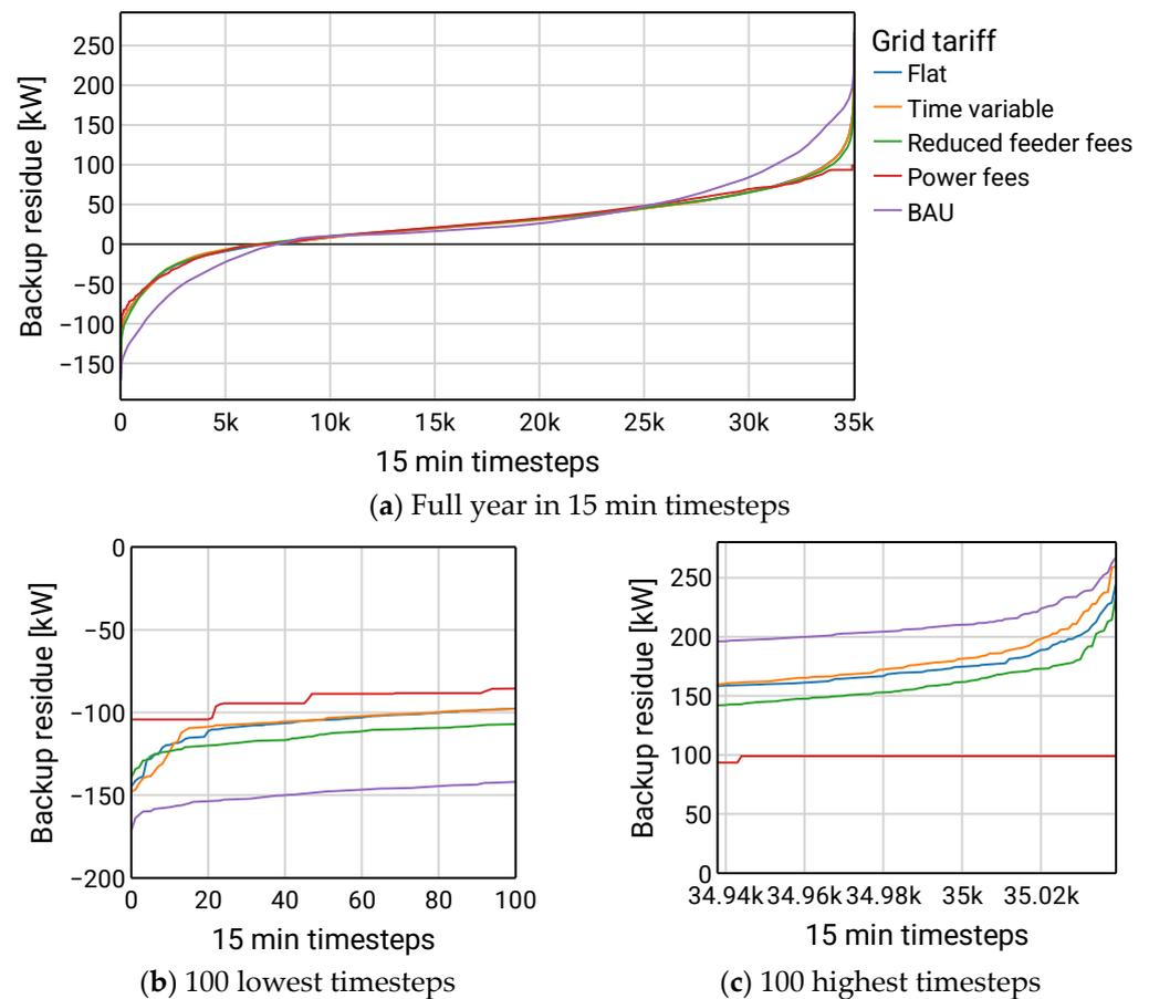
**Figure 8.** Load duration curves for a variation of grid tariff scenarios for a full simulation year (a), the 100 timesteps with lowest residual load (b) and the highest residual load (c). Data from scenario year 2035 and the rural distribution grid.
