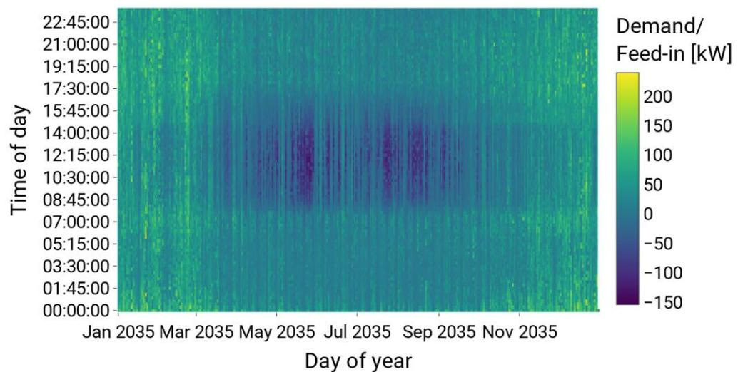
**Figure A3.** Heatmap of the electric demand (positive values) and feed-in (negative values) for the feeder fee scenario, the scenario year 2035 and the rural grid.
