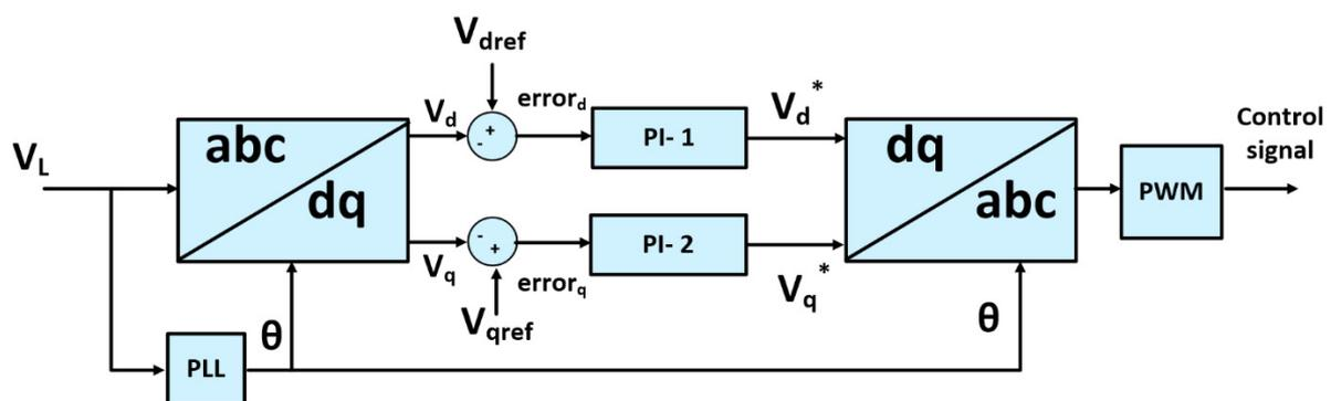
Figure 3. DVR control block diagram.
