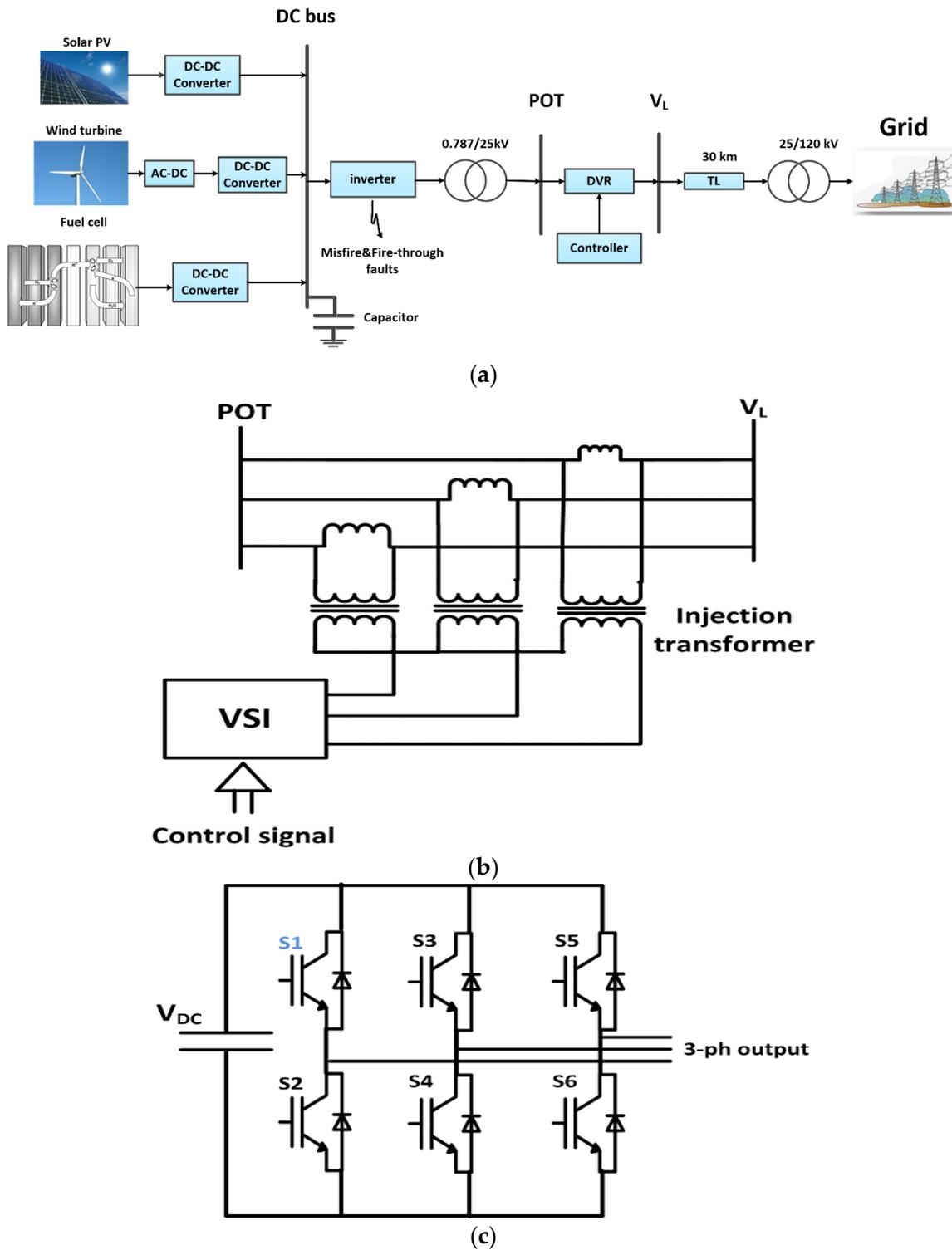
Figure 1. System under study. (a)—Hybrid power system, (b)—DVR, (c)—The main circuit of the 3-ph inverter.
