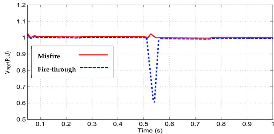
**Figure 5.** Point of Common Coupling (POT) voltage.
