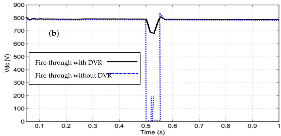
**Figure 9.** POT and DC link voltage during fire-through fault with and without using DVR. (a)—POT voltage, (b)—DC link voltage.
