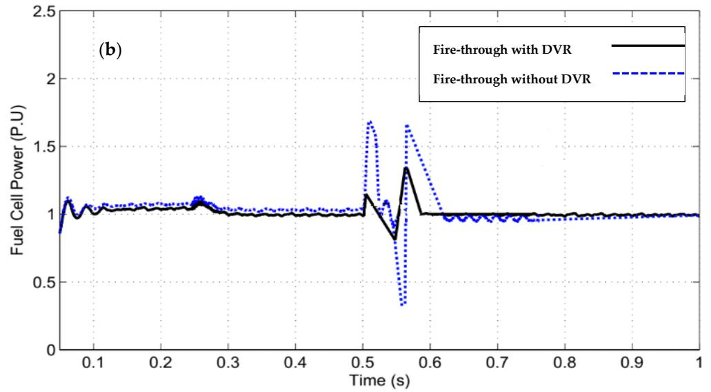
Figure 10. PV and FC power during fire-through faults while using DVR. (a)—PV, (b)—FC.
