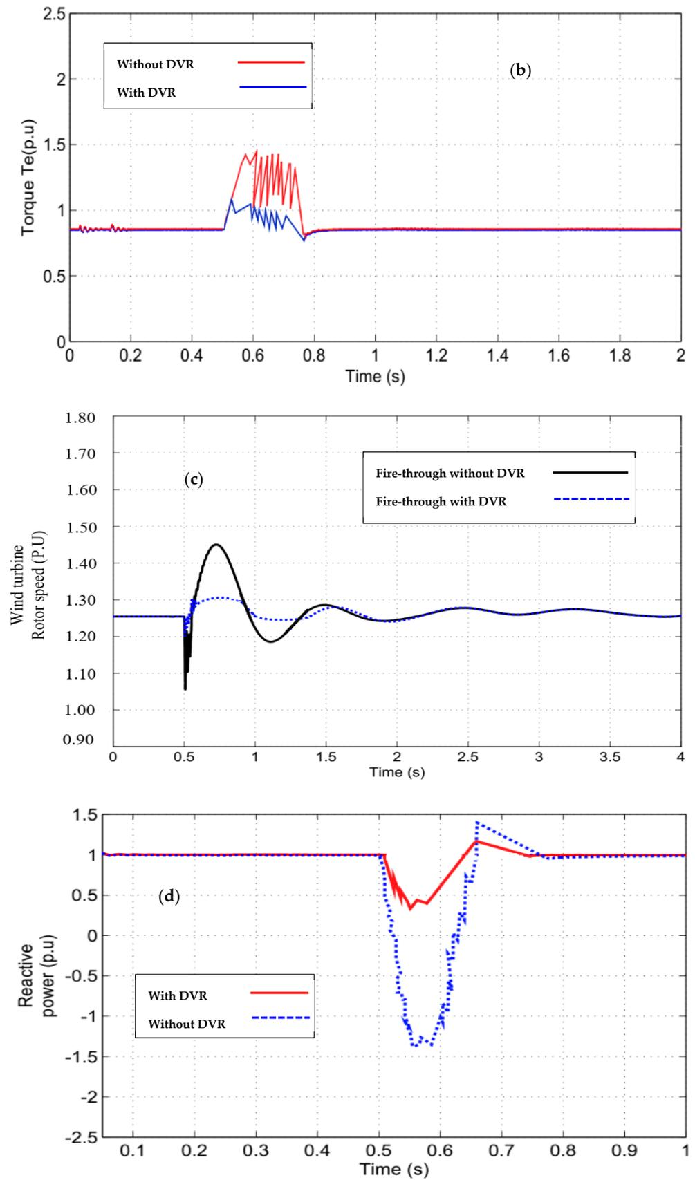
**Figure 11.** WECS efficacy during faults. (a)—power, (b)—torque, (c)—wind rotor speed, (d)—reactive power.
