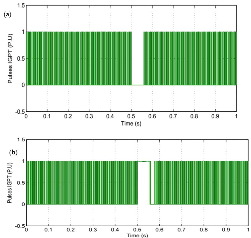
**Figure 4.** Intermittent faults at S1 of the inverter. (a)—Misfire fault, (b)—Fire-through fault.
