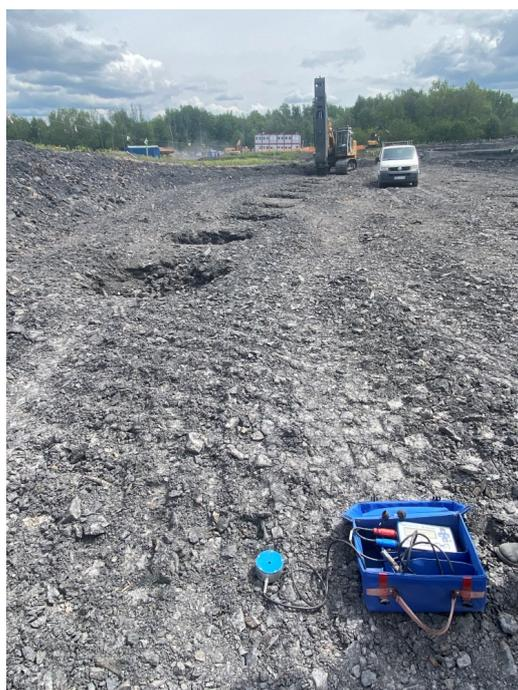
**Figure 20.** First stage of vibration control—safe distance from formworks (by J. Rybak).
