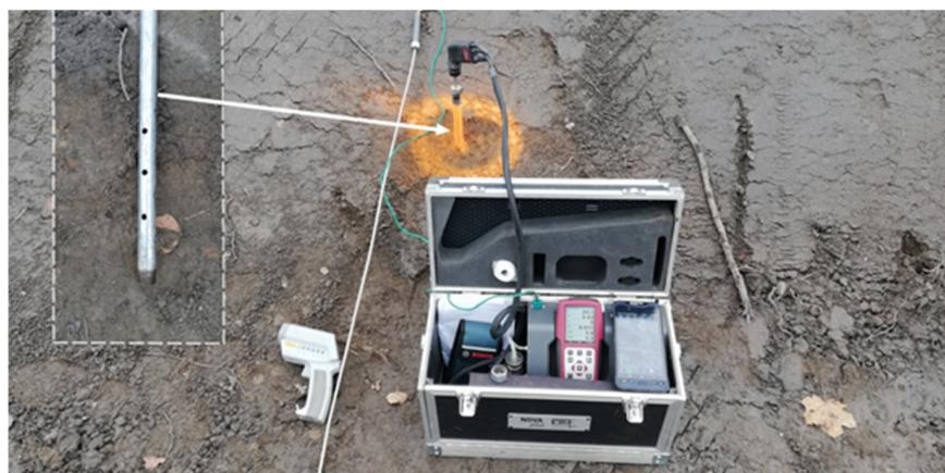
**Figure 14.** Measurement point as part of thermal condition monitoring (own elaboration).
