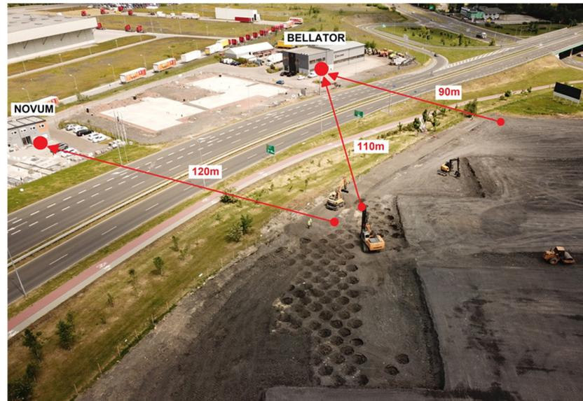
**Figure 21.** Vibration measurement area—control of the influence on the gabions' substrate (graphic by P. Dobrzycki).
