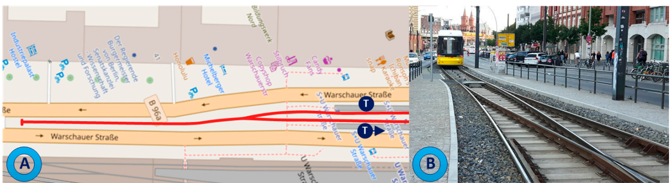
Figure 5. Terminating a tram route without applying a tram loop—Warsaw Street, Berlin, Germany: (A) own study based on openstreetmap.org; (B) own study.
