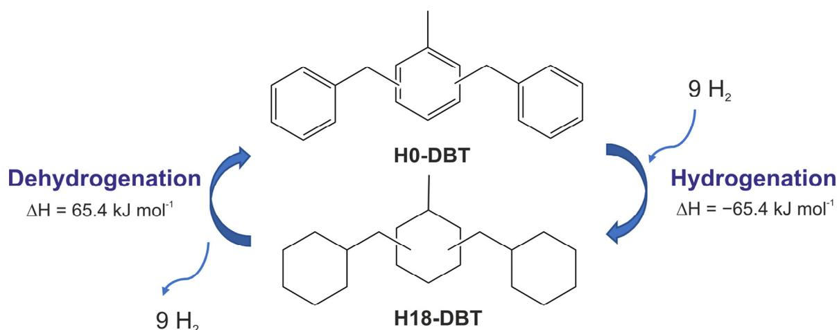
**Figure 3.** Schematic representation of reversible hydrogen storage by H0-DBT/H18-DBT system.
