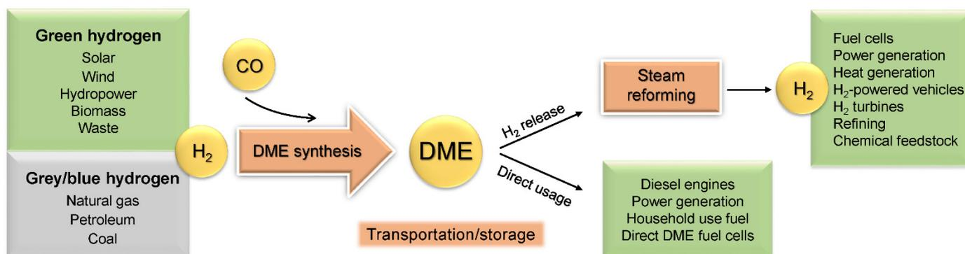
**Figure 1.** Schematic route of DME synthesis, transportation, and utilization.
