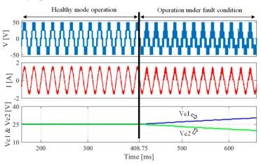
Figure 3. Simulation results of the inverter operation under open-circuit fault occurrence in  $D_{C4}$ , without fault-tolerant strategy.
