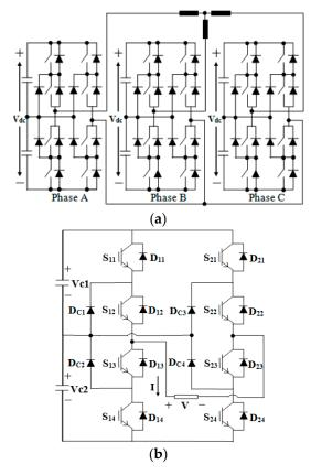
**Figure 1.** Scheme of (**a**) a three-phase five-level NPC/H-bridge inverter, and (**b**) a single-phase five-level NPC inverter.
