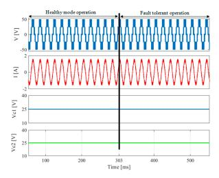
Figure 7. Simulation results for fault-tolerant operation of the inverter in case of fault occurrence in S<sub>11</sub>.
