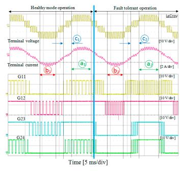
Figure 12. Detailed experimental results of the fault-tolerant strategy in case of fault event in D<sub>c4</sub>.
