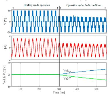
**Figure 6.** Simulation results of the inverter operation under open-circuit fault occurrence in  $S_{11}$ , without fault-tolerant strategy.
