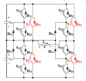
Figure 2. Proposed fault-tolerant topology.
