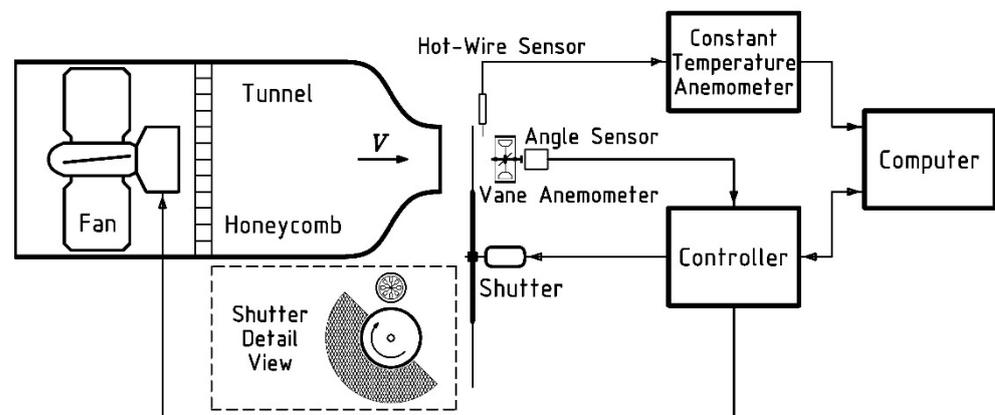
**Figure 1.** Diagram of the test stand.
