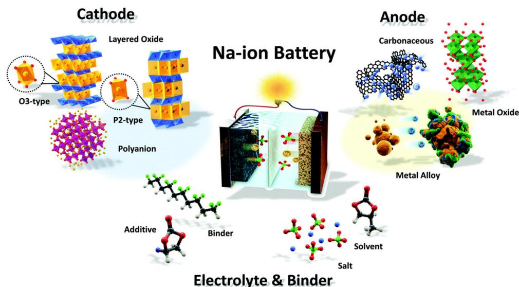
**Figure 4.** Schematic of the structure and illustration of a Na-ion battery system. Adapted with permission [15]. Copyright (2017) Royal Society of Chemistry. This article is an open access article distributed under the terms and conditions of the Creative Commons Attribution (CC BY) license.
