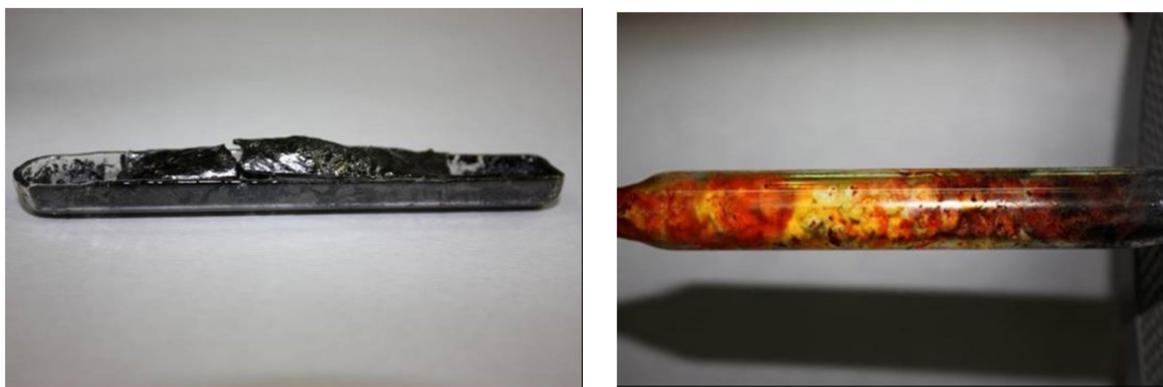
**Figure 15.** Quartz boat and reactor tube after pyrolysis of RW in tubular reactor at 600 °C.
