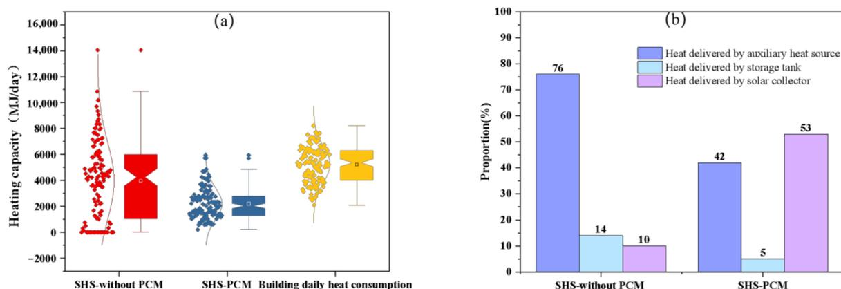
**Figure 10.** (a) Daily heat delivered by the AHS of the SHS-PCM and the SHS-without PCM, as well as daily heat consumption of the building; (b) the proportion of heat delivered by AHS, heat storage tank, and solar collector in the SHS-without PCM and the SHS-PCM.
