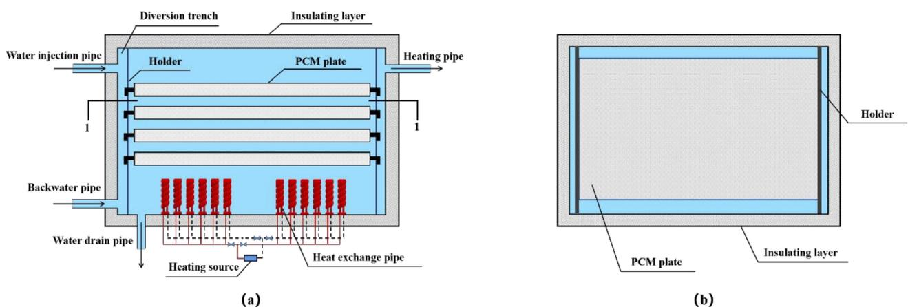
**Figure 1.** (a) Front view of the PCM storage tank; (b) 1-1 cross sectional of the PCM storage tank.
