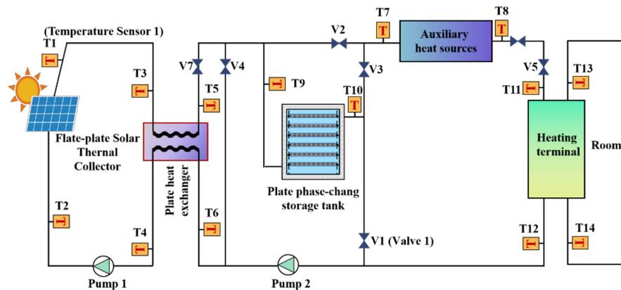
**Figure 9.** Schematic diagram of composite solar phase change heat storage combined with air-cooled heat pump heating system.
