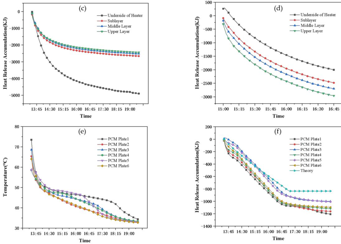
**Figure 7.** In working condition 2: (a) Water temperature curve of the PCM storage tank; (b) Water temperature curve of the common tank; (c) Heat release accumulation curve of the PCM storage tank; (d) Heat release accumulation curve of the common tank; (e) Temperature curve of the PCM plate; (f) Heat release accumulation curve of the PCM plate.
