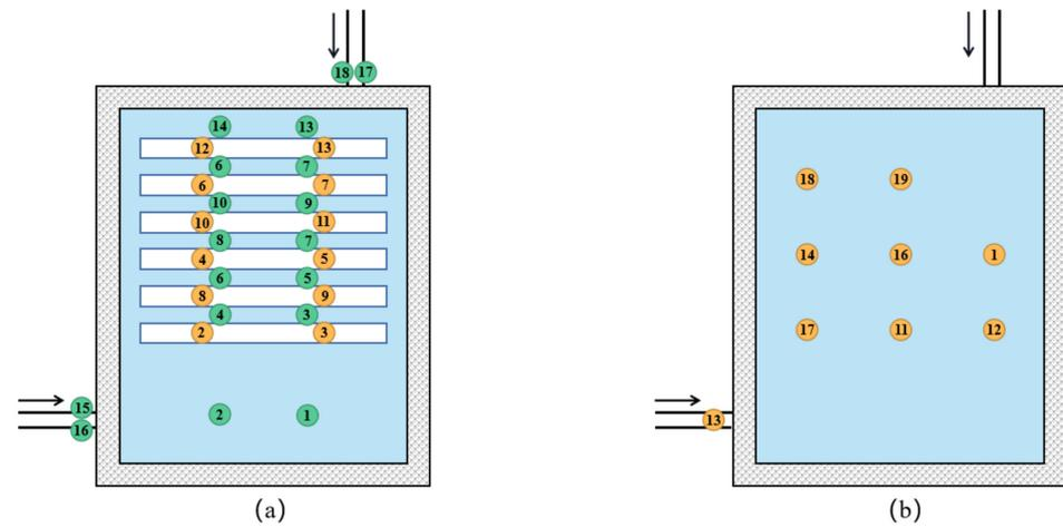
**Figure 5.** (a) Test points of temperature in the PCM storage tank; (b) Test points of temperature in the common tank.
