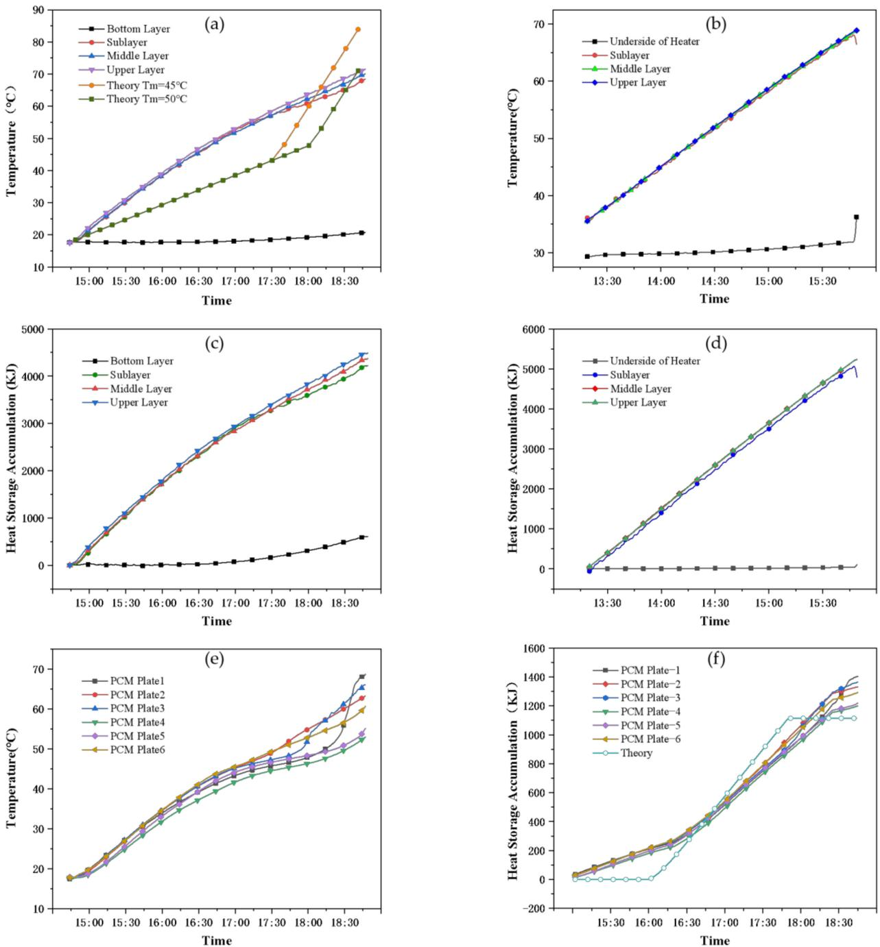
**Figure 6.** In working condition 1: (a) Water temperature curve of the PCM storage tank; (b) Water temperature curve of the common tank; (c) Heat storage accumulation curve of the PCM storage tank; (d) Heat storage accumulation curve of the common tank; (e) Temperature curve of the PCM plate; (f) Heat storage accumulation curve of the PCM plate.
