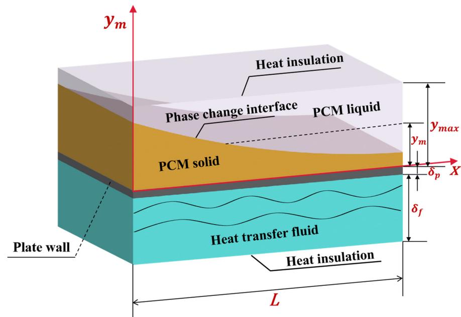
**Figure 2.** Mathematical model of phase change heat storage unit.
