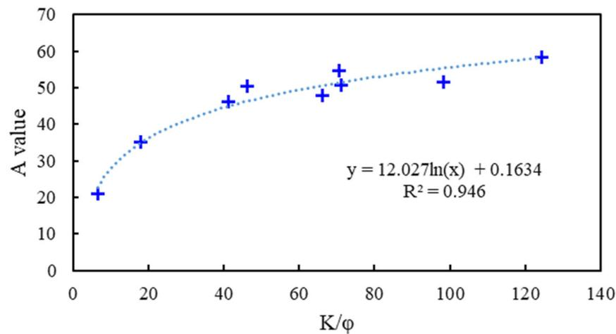
Figure 7. The relationship between the value of coefficient A and the ratio of  $k/\varphi$ .
