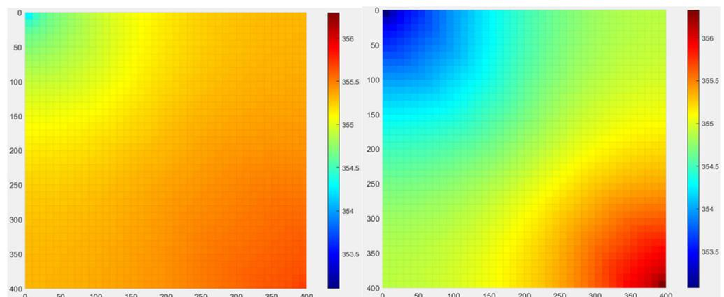
**Figure 11.** The water saturation distribution at the 50th time step (the left is the numerical simulation results considering the relative permeability of high waterflooding PVs, and the right is the traditional numerical simulation results).
