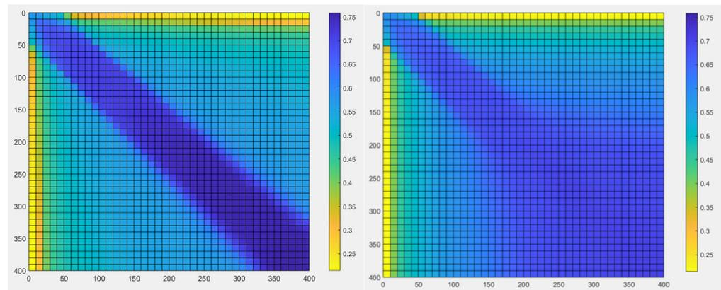
**Figure 10.** The water saturation distribution at the 50th time step (The left is the numerical simulation results considering the relative permeability of high waterflooding PVs, and the right is the traditional numerical simulation results).
