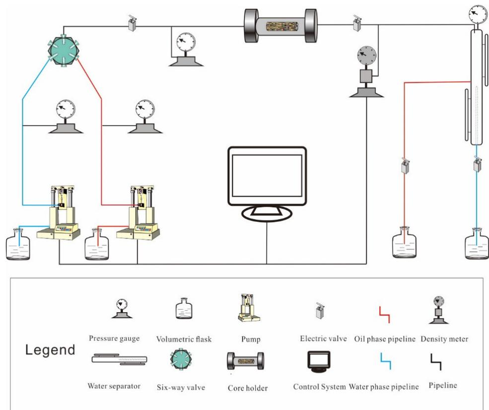
**Figure 2.** Schematic representation of the experimental apparatus of the relative permeability measurement.
