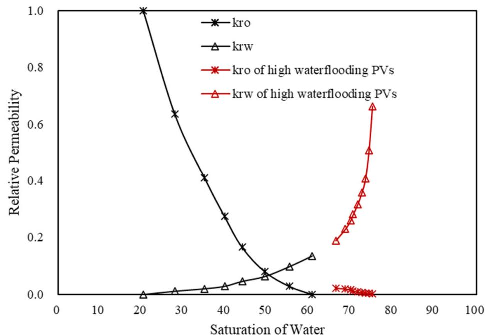
Figure 3. Relative permeability curve of #4 ( $K = 1793.1$  mD).
