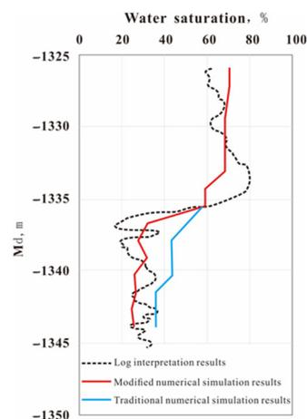
**Figure 13.** The comparison between the actual logging interpretation oil saturation curve and the model oil saturation curve of a passing well.
