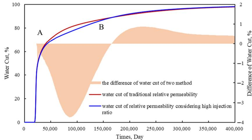
**Figure 12.** The water cut curve of numerical simulation of traditional simulator and simulator that considering high water waterflooding PVs.
