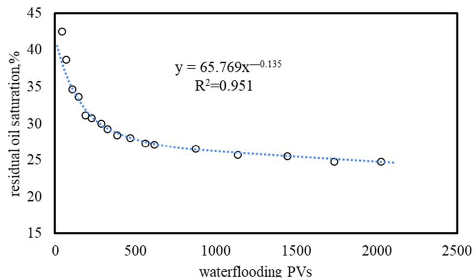
**Figure 6.** The relationship between the waterflooding PVs and the residual oil saturation.
