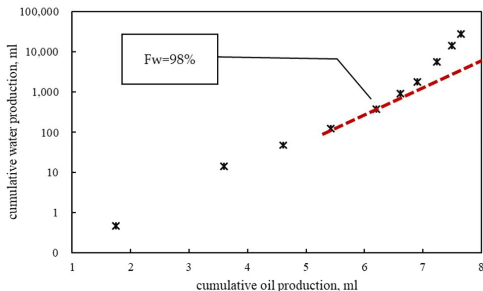
**Figure 4.** Type A waterflood characteristic curve of #4.
