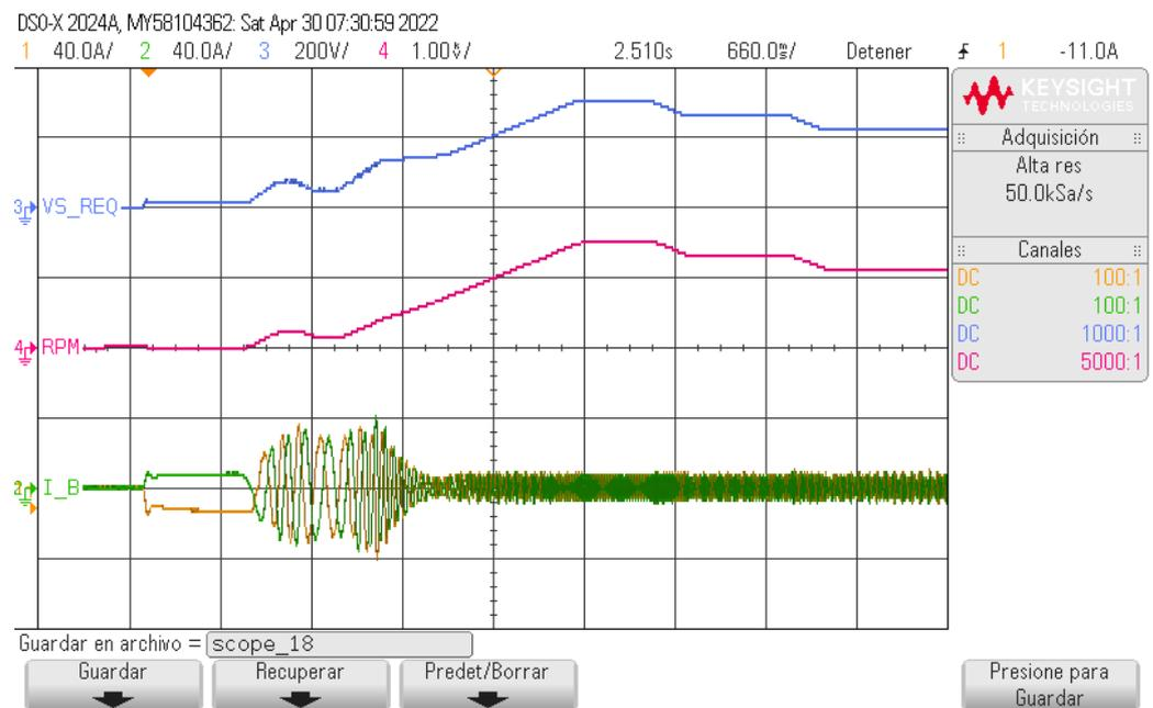
**Figure 5.** Oscilloscope waveforms of  $V_s^*$ ,  $\omega_r$ , and  $i_a$  and  $i_b$ , for the previous HST-SCS [17].
