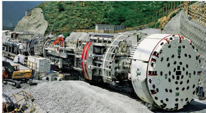
**Figure 4.** The earth pressure balance shield TBM used.
