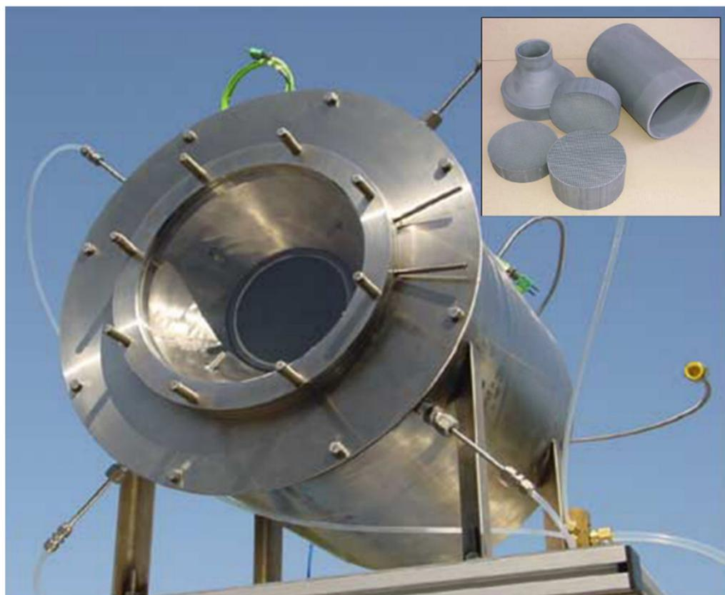
**Figure 7.** The HYDROSOL solar receiver-reactor used for water splitting showing the installment position and configuration of Mn/Zn-ferrite coated SiC honeycombs [141].
