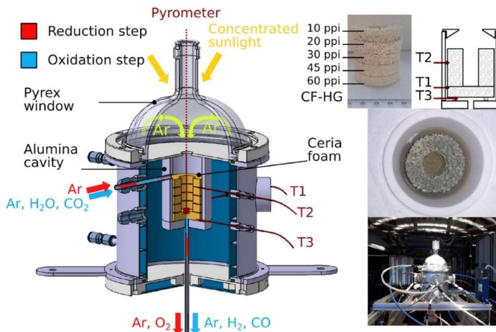
**Figure 13.** Schematic of the  $1.5\text{-kW}_{\text{th}}$  directly irradiated solar reactor equipped with a series of ceria RPCs with 10–60-ppi gradient pore sizes used for  $\text{H}_2\text{O}$  or  $\text{CO}_2$  splitting [73].
