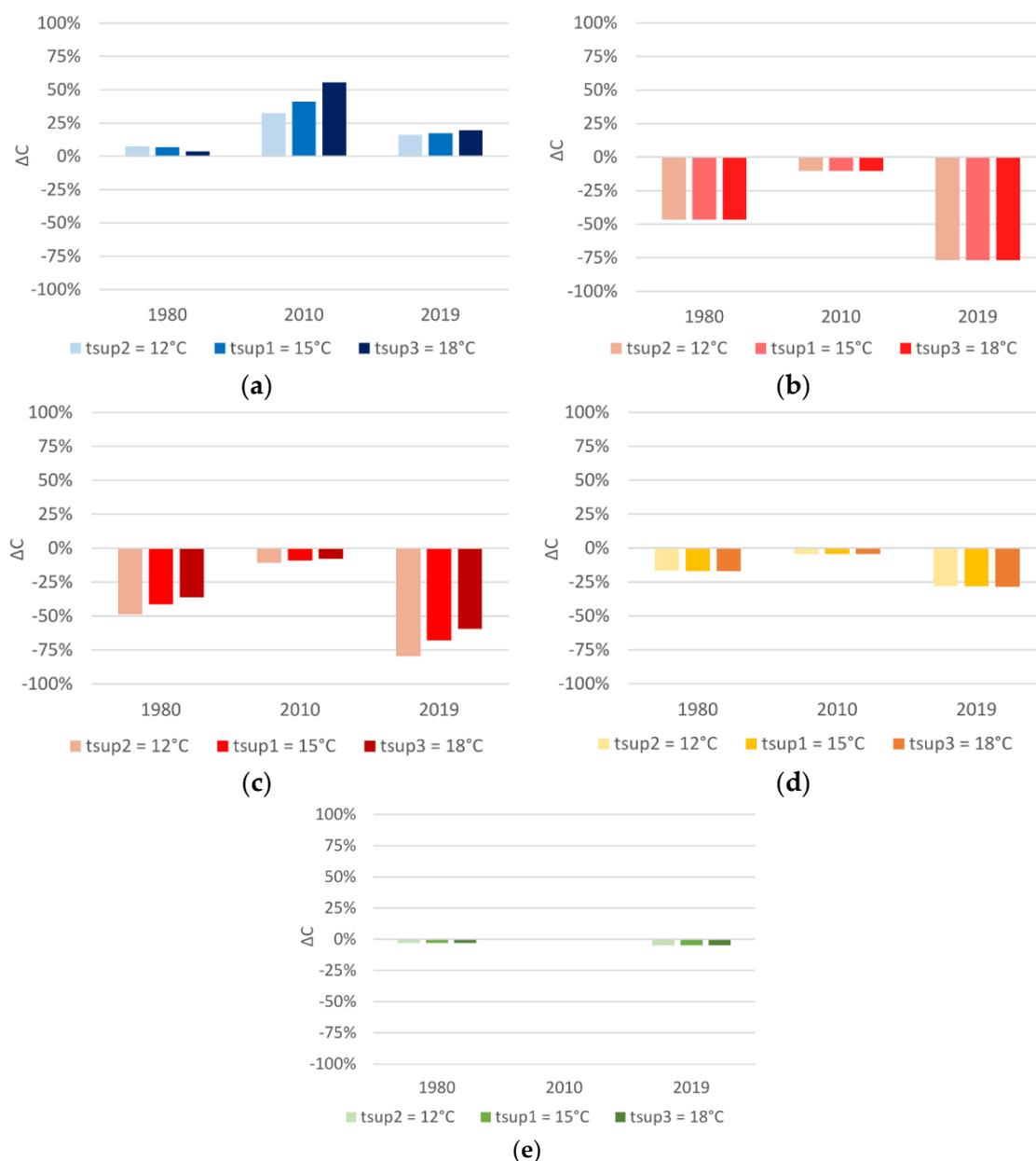
**Figure 17.** Relative capacity of heat exchangers, compared to 1969: (a) cooler, (b) preheater, (c) heater, (d) humidifier, (e) and plate heat exchanger.
